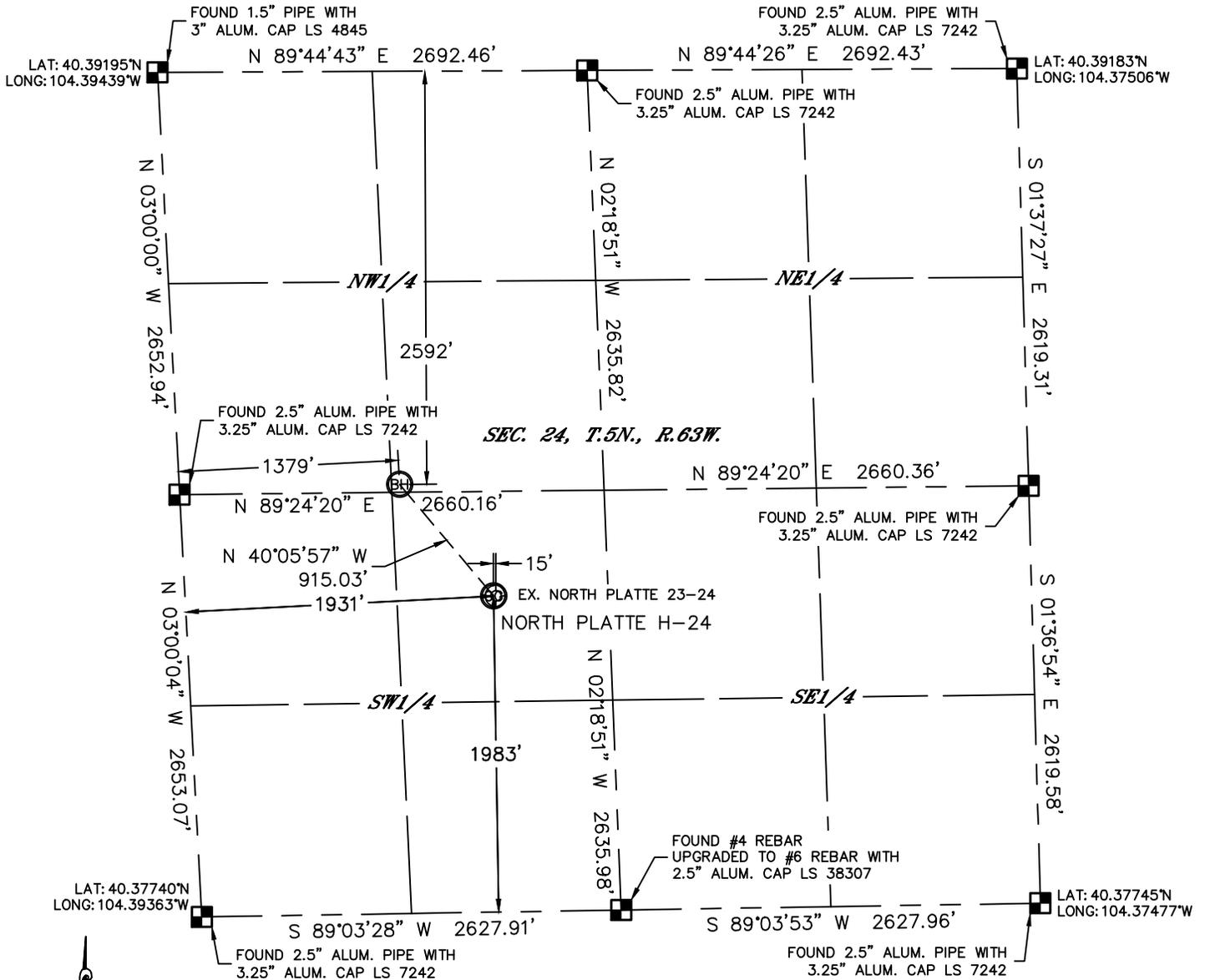
In accordance with a request from KEITH CAPLAN with BONANZA CREEK ENERGY, INC. Lat40°, Inc. has determined the surface location of the NORTH PLATTE H-24 to be 1983' from the SOUTH line and 1931' from the WEST line and the bottom hole to be 2592' from the NORTH line and 1379' from the WEST line as measured at right angles from the section lines of Section 24, Township 5 North, Range 63 West of the Sixth Principal Meridian, County of Weld, State of Colorado.
