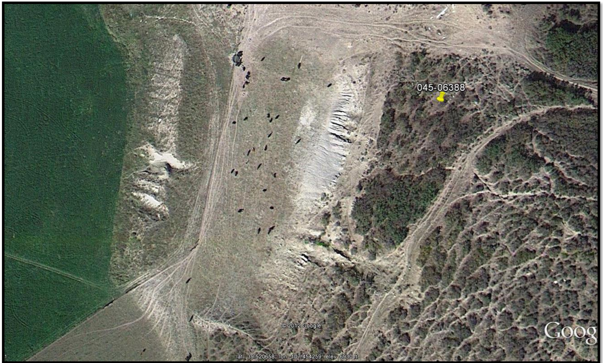
Google Maps Aerial Photo Date: September 22, 2011. Aerial view of the Snyder-Barton-Porter 2-21 location. Showing rills and gully on cut and fill slopes.
