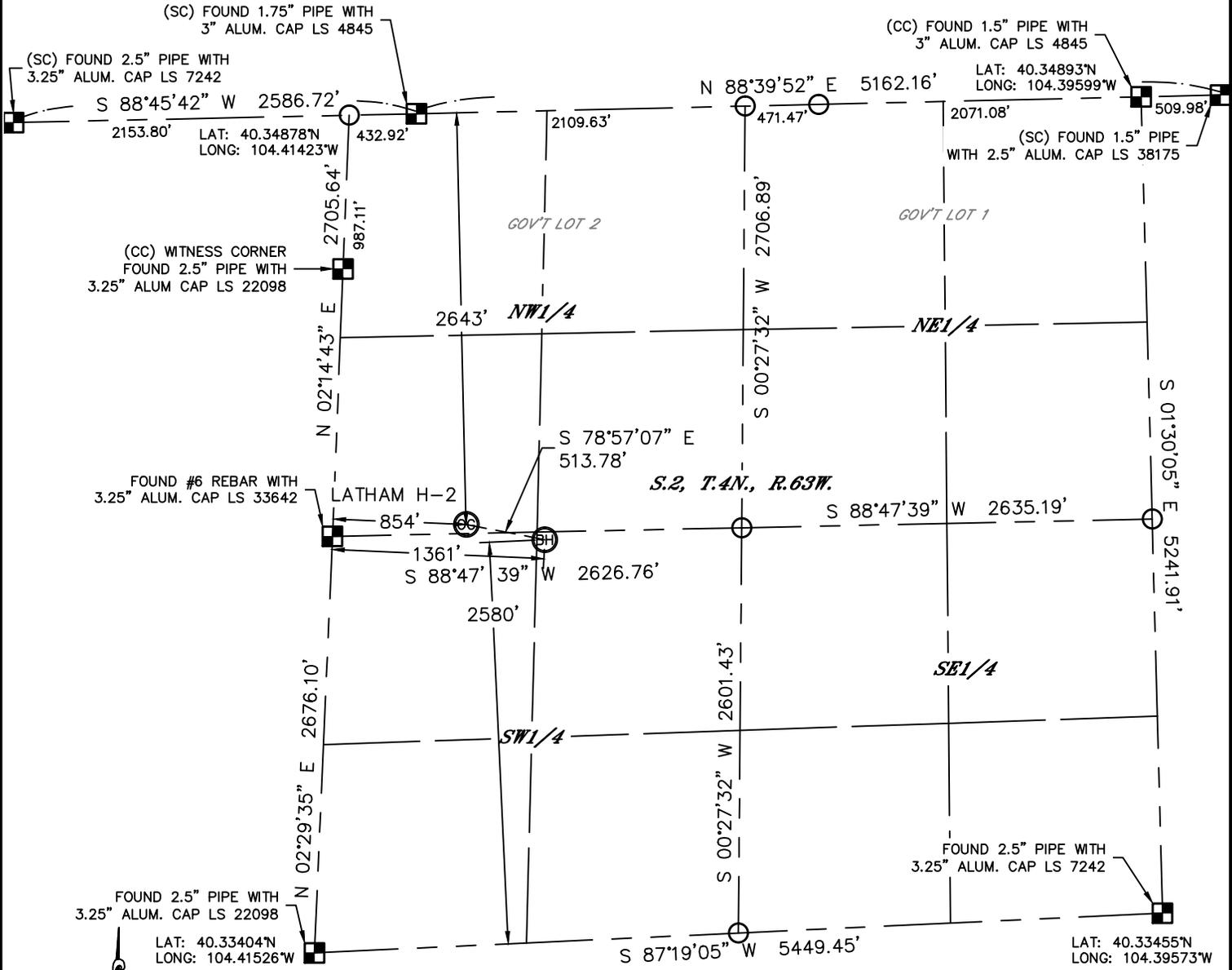
In accordance with a request from Keith Caplan with BONANZA CREEK ENERGY, INC. Lat40°, Inc. has determined the surface location of the LATHAM H-2 to be 2643' from the NORTH line and 854' from the WEST line and the bottom hole to be 2580' from the SOUTH line and 1361' from the WEST line as measured at right angles from the section lines of Section 2, Township 4 North, Range 63 West of the Sixth Principal Meridian, County of Weld, State of Colorado.
