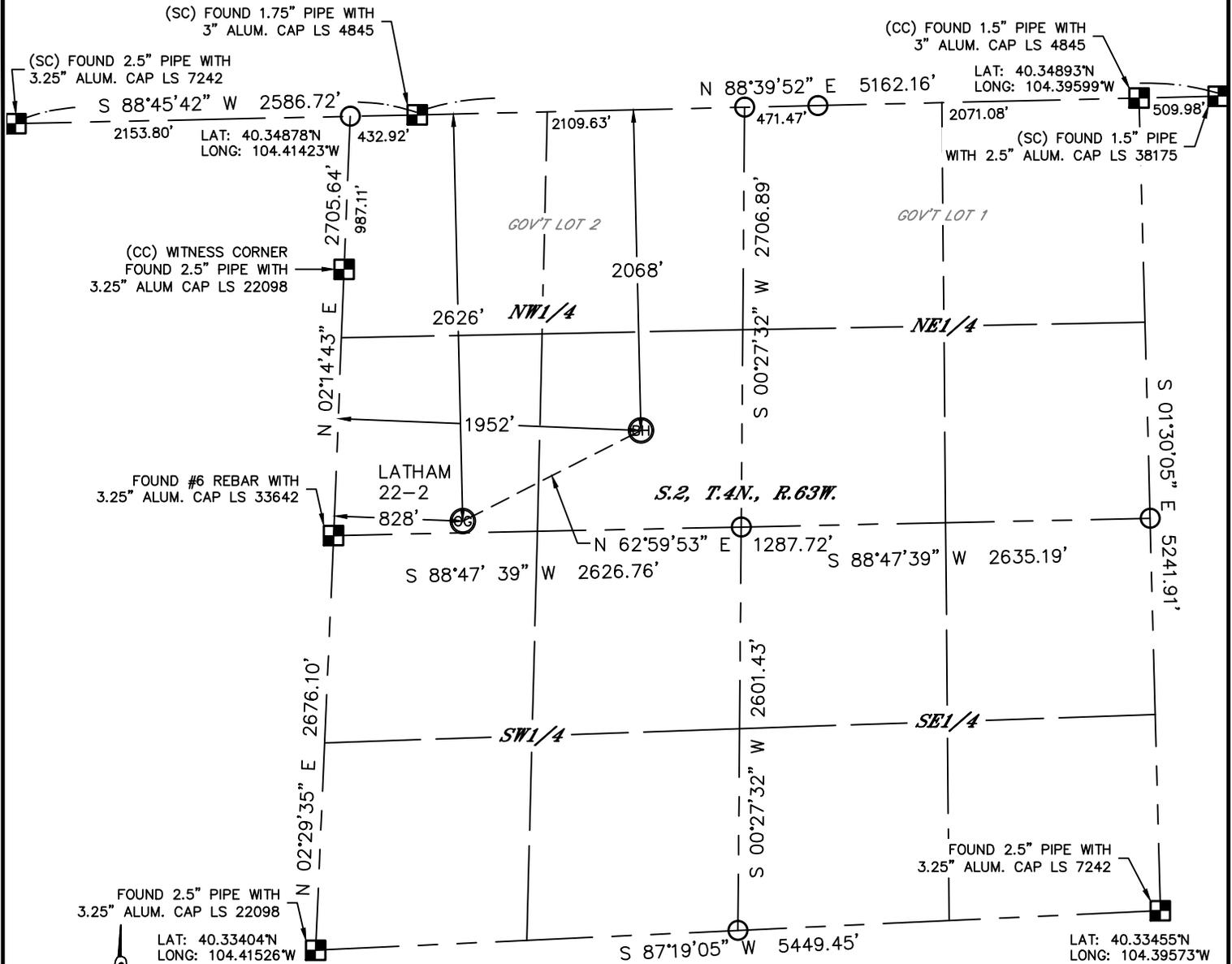
In accordance with a request from Keith Caplan with BONANZA CREEK ENERGY, INC. Lat40°, Inc. has determined the surface location of the LATHAM 22-2 to be 2626' from the NORTH line and 828' from the WEST line and the bottom hole to be 2068' from the NORTH line and 1952' from the WEST line as measured at right angles from the section lines of Section 2, Township 4 North, Range 63 West of the Sixth Principal Meridian, County of Weld, State of Colorado.
