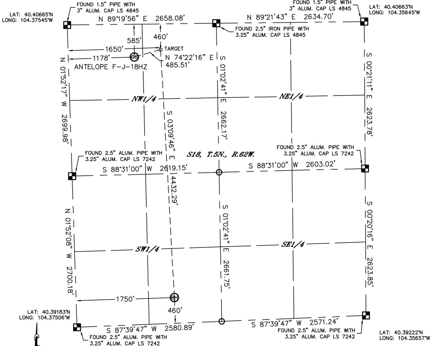
In accordance with a request from Keith Caplan with BONANZA CREEK ENERGY, INC. Lat40°, Inc. has determined the surface location of the ANTELOPE F-J-18HZ to be 585' from the NORTH line and 1178' from the WEST line and the bottom hole to be 460' from the SOUTH line and 1750' from the WEST line as measured at right angles from the section lines of Section 18, Township 5 North, Range 62 West of the Sixth Principal Meridian, County of Weld, State of Colorado.
