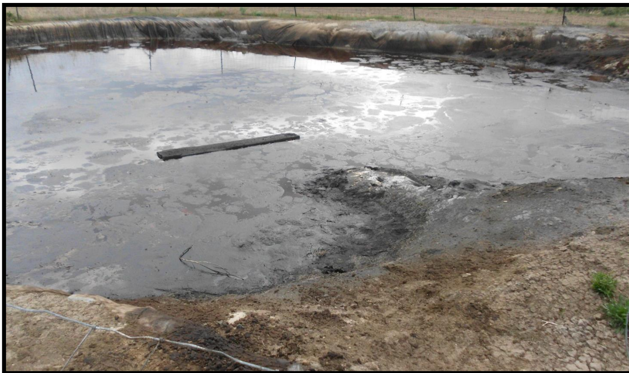
View of larger pit: (northeast of smaller secondary pit) oil and condensate accumulation at pit surface . Approx. 40' x 60'
