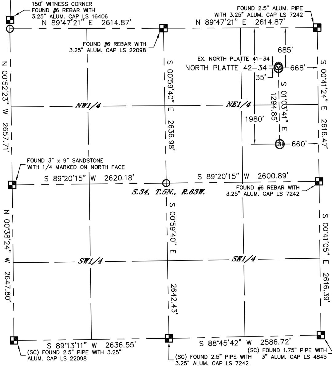
In accordance with a request from Keith Caplan with BONANZA CREEK ENERGY, INC. Lat40°, Inc. has determined the surface location of the NORTH PLATTE 42-34 to be 685' from the NORTH line and 668' from the EAST line and the bottom hole to be 1980' from the NORTH line and 660' from the EAST line as measured at right angles from the section lines of Section 34, Township 5 North, Range 63 West of the Sixth Principal Meridian, County of Weld, State of Colorado.
