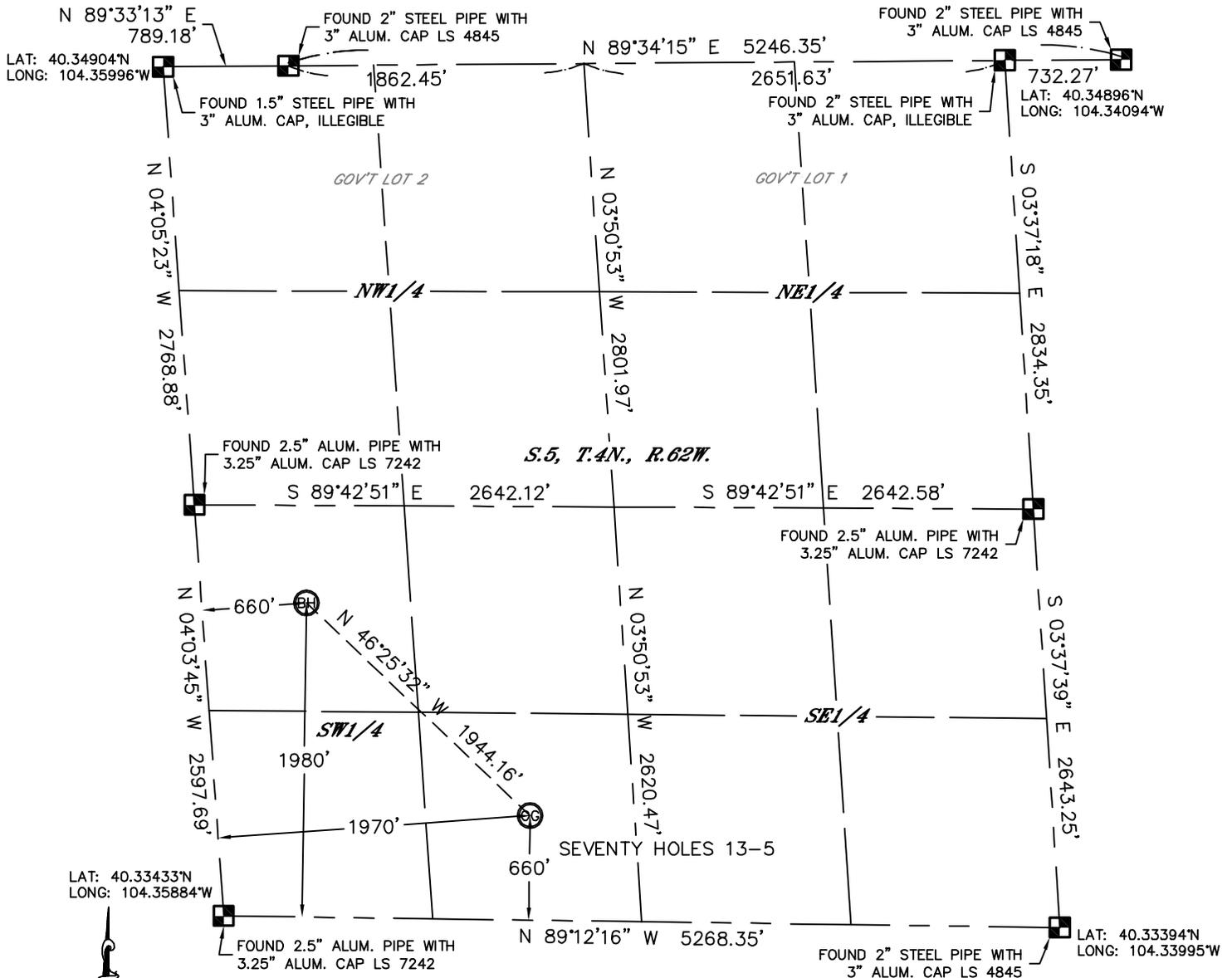
In accordance with a request from Keith Caplan with BONANZA CREEK ENERGY, INC. Lat40°, Inc. has determined the surface location of the SEVENTY HOLES 13-5 to be 660' from the SOUTH line and 1970' from the WEST line and the bottom hole to be 1980' from the SOUTH line and 660' from the WEST line as measured at right angles from the section lines of Section 5, Township 4 North, Range 62 West of the Sixth Principal Meridian, County of Weld, State of Colorado.
