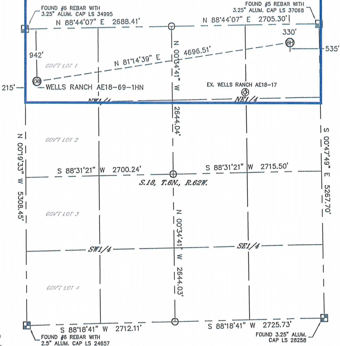
In accordance with a request from Sean Casper with Noble Energy Inc. Lat40°, Inc. has determined the surface location of the WELLS RANCH AE18-69-1HN to be 942' from the NORTH line and 215' from the WEST line and the bottom hole to be 330' from the NORTH line and 535' from the EAST line as measured at right angles from the section lines of Section 18, Township 6 North, Range 62 West of the Sixth Principal Meridian, County of Weld, State of Colorado.
