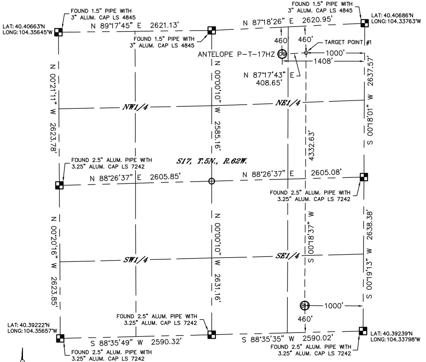
In accordance with a request from Keith Caplan with BONANZA CREEK ENERGY, INC. Lat40°, Inc. has determined the surface location of the ANTELOPE P-T-17HZ to be 460' from the NORTH line and 1408' from the EAST line and the bottom hole to be 460' from the SOUTH line and 1000' from the EAST line as measured at right angles from the section lines of Section 17, Township 5 North, Range 62 West of the Sixth Principal Meridian, County of Weld, State of Colorado.
