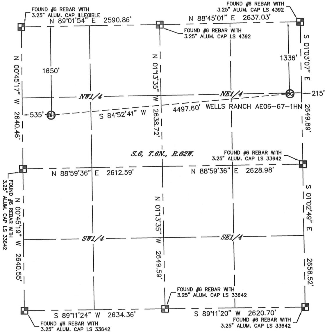
In accordance with a request from Sean Casper with Noble Energy Inc. Lat40°, Inc. has determined the surface location of the WELLS RANCH AE06-67-1HN to be 1336' from the NORTH line and 215' from the EAST line and the bottom hole to be 1650' from the NORTH line and 535' from the WEST line as measured at right angles from the section lines of Section 6, Township 6 North, Range 62 West of the Sixth Principal Meridian, County of Weld, State of Colorado.
