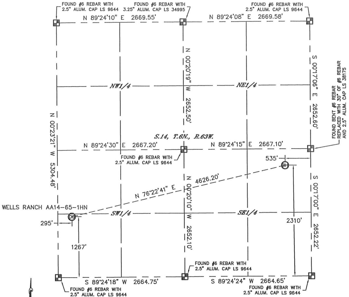
In accordance with a request from Sean Casper with Noble Energy Inc. Lat40°, Inc. has determined the surface location of the WELLS RANCH AA14-65-1HN to be 1267' from the SOUTH line and 295' from the WEST line and the bottom hole to be 2310' from the SOUTH line and 535' from the EAST line as measured at right angles from the section lines of Section 14, Township 6 North, Range 63 West of the Sixth Principal Meridian, County of Weld, State of Colorado.
