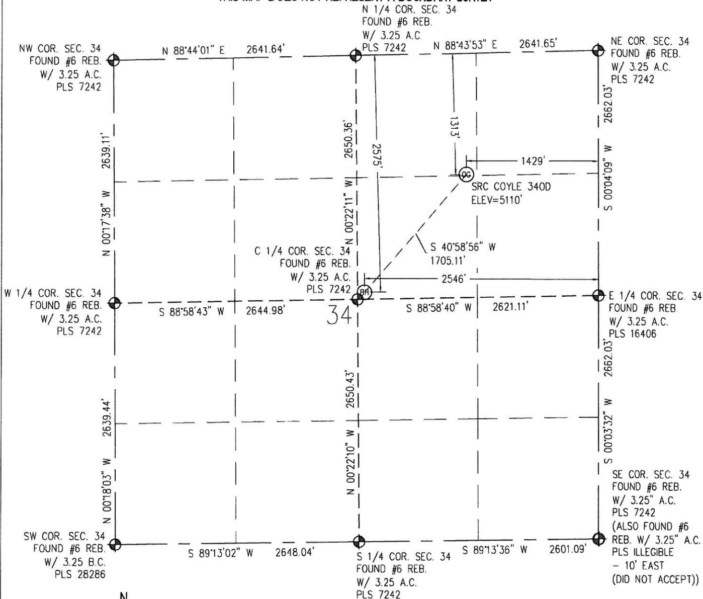
IN ACCORDANCE WITH A REQUEST FROM CRAIG RASMUSON - SYNERGY RESOURCES, BASELINE ENGINEERING CORP. HAS DETERMINED THE LOCATION OF THE SRC COYLE 340D TO BE 1,313' FNL AND 1,429' FEL, AS MEASURED AT NINETY (90) DEGREES FROM THE SECTION LINE OF SECTION 34, TOWNSHIP 4 NORTH, RANGE 68 WEST AND THE BOTTOM HOLE LOCATION TO BE 2,575' FNL AND 2,546' FEL OF SECTION 34, TOWNSHIP 4 NORTH, RANGE 68 WEST, 6TH PRINCIPAL MERIDIAN, WELD COUNTY, COLORADO.
