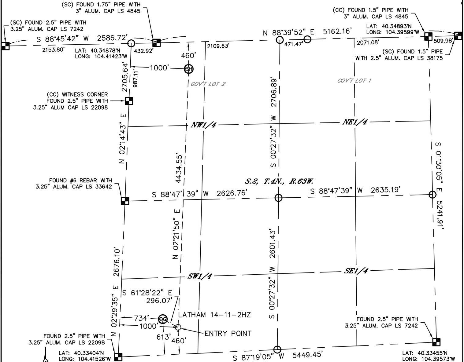
In accordance with a request from Keith Caplan with BONANZA CREEK ENERGY, INC. Lat40°, Inc. has determined the surface location of the LATHAM 14-11-2HZ to be 613' from the SOUTH line and 734' from the WEST line and the bottom hole to be 460' from the NORTH line and 1000' from the WEST line as measured at right angles from the section lines of Section 2, Township 4 North, Range 63 West of the Sixth Principal Meridian, County of Weld, State of Colorado.
