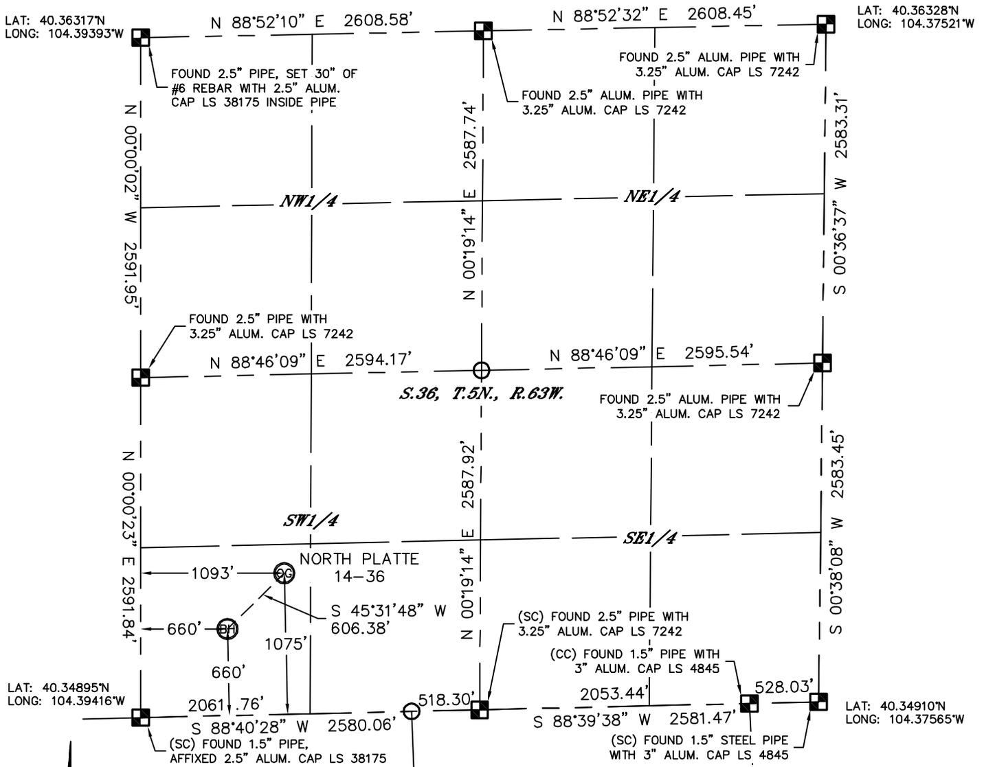
In accordance with a request from Keith Caplan with BONANZA CREEK ENERGY, INC. Lat40°, Inc. has determined the surface location of the NORTH PLATTE 14-36 to be 1075' from the SOUTH line and 1093' from the WEST line and the bottom hole to be 660' from the SOUTH line and 660' from the WEST line as measured at right angles from the section lines of Section 36, Township 5 North, Range 63 West of the Sixth Principal Meridian, County of Weld, State of Colorado.
