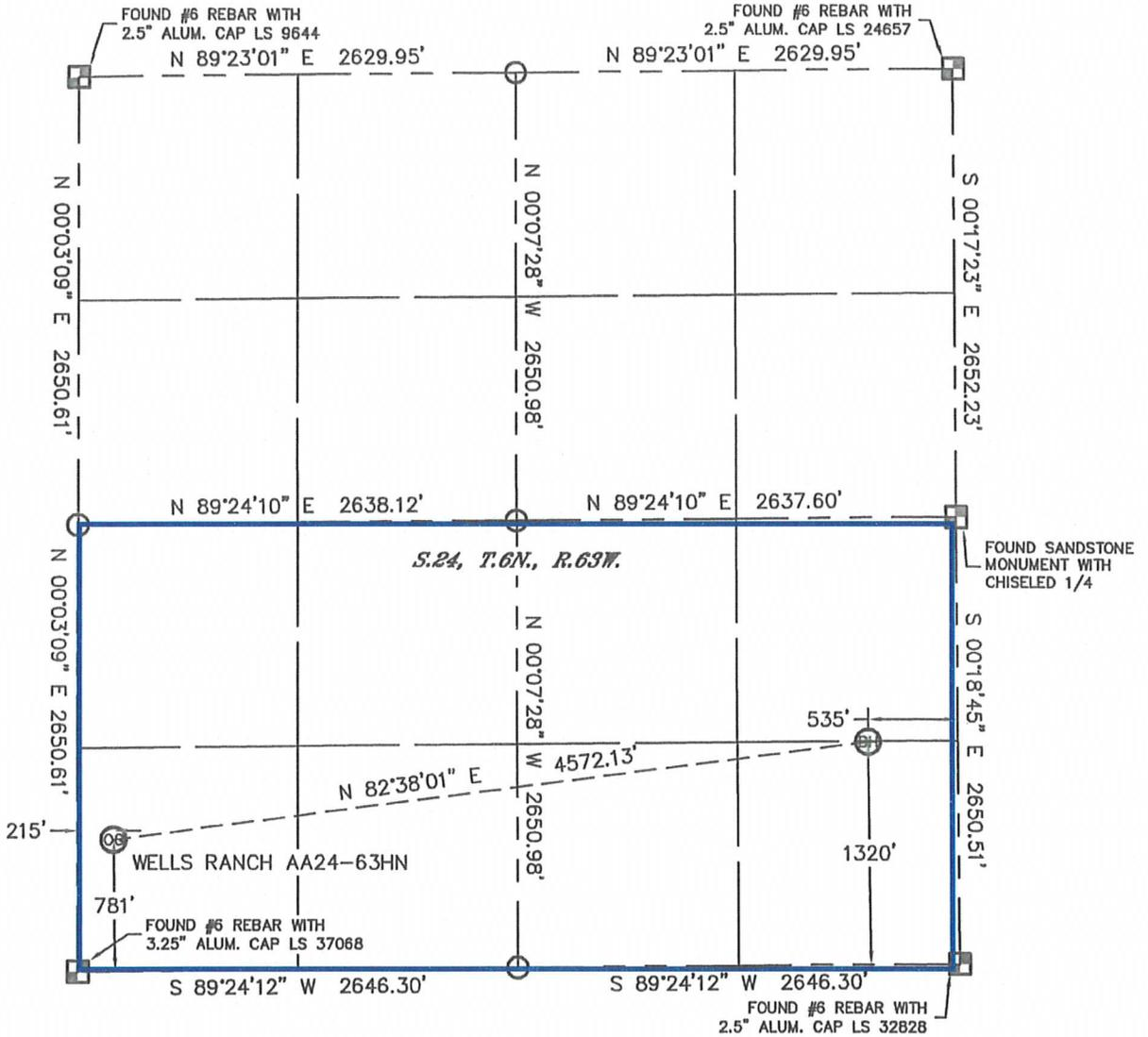
In accordance with a request from Sean Casper with Noble Energy Inc. Lat40°, Inc. has determined the surface location of the WELLS RANCH AA24-63HN to be 781' from the SOUTH line and 215' from the WEST line and the bottom hole to be 1320' from the SOUTH line and 535' from the EAST line as measured at right angles from the section lines of Section 24, Township 6 North, Range 63 West of the Sixth Principal Meridian, County of Weld, State of Colorado.
