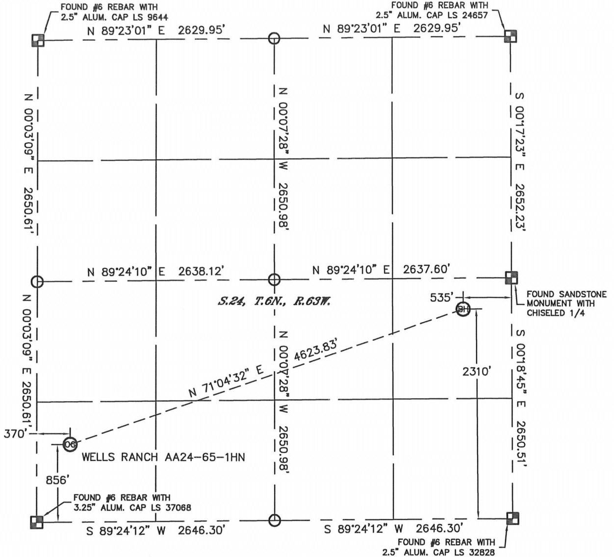
In accordance with a request from Sean Casper with Noble Energy Inc., Lat40°, Inc. has determined the surface location of the WELLS RANCH AA24-65-1HN to be 856' from the SOUTH line and 370' from the WEST line and the bottom hole to be 2310' from the SOUTH line and 535' from the EAST line as measured at right angles from the section lines of Section 24, Township 6 North, Range 63 West of the Sixth Principal Meridian, County of Weld, State of Colorado.
