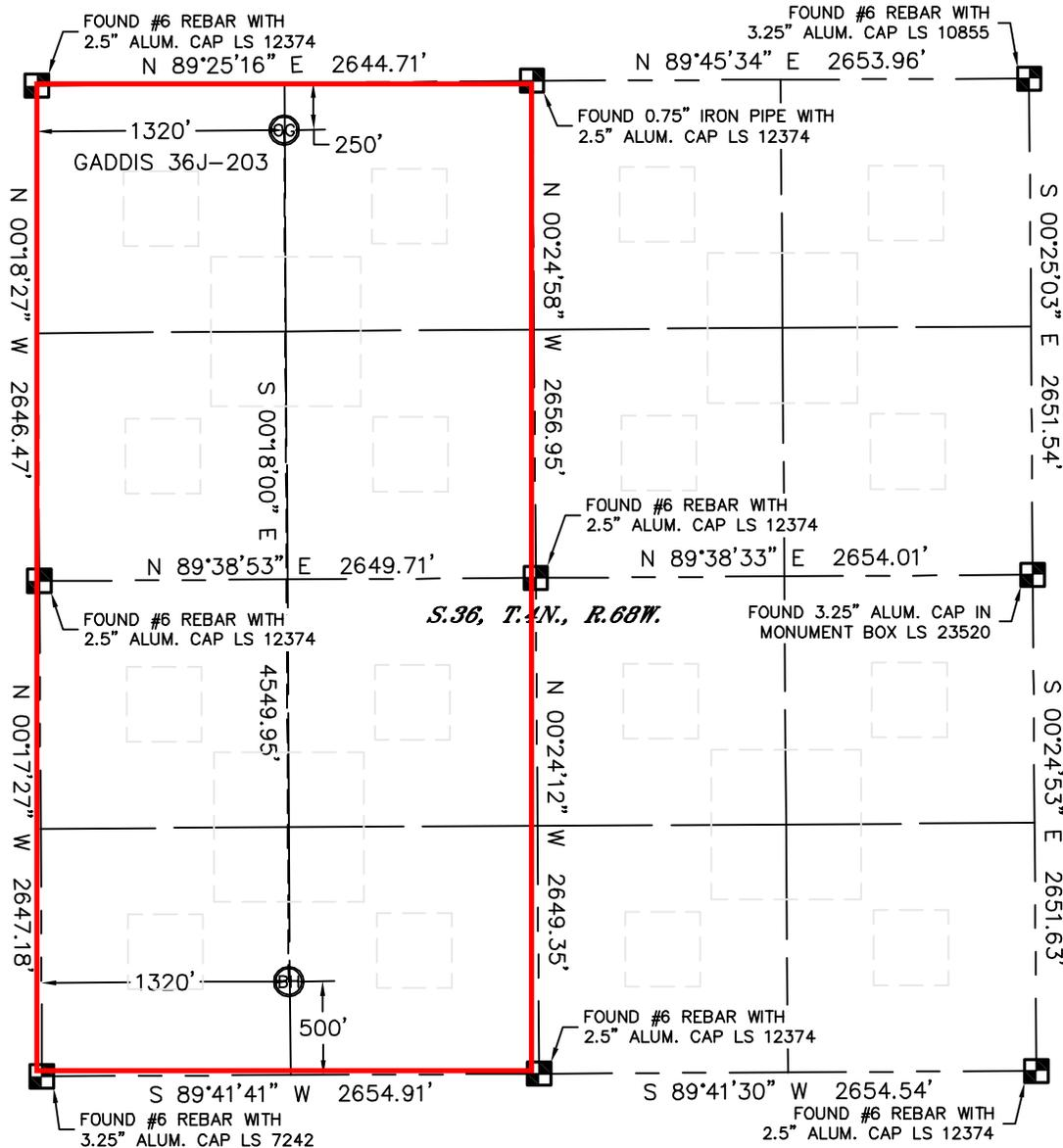
In accordance with a request from Mac Neumann with PDC ENERGY Lat40°, Inc. has determined the surface location of the GADDIS 36J-203 to be 250' from the NORTH line and 1320' from the WEST line and the bottom hole to be 500' from the SOUTH line and 1320' from the WEST line as measured at right angles from the section lines of Section 36, Township 4 North, Range 68 West of the Sixth Principal Meridian, County of Weld, State of Colorado.
