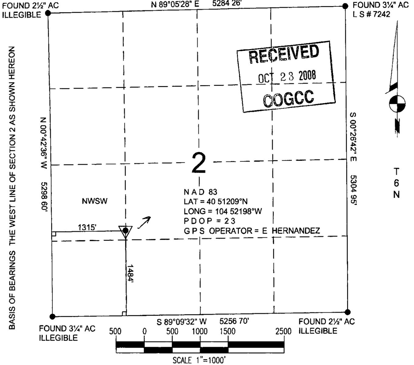
POWER SURVEYING COMPANY, INC OF FREDERICK, COLORADO HAS IN ACCORDANCE WITH A REQUEST FROM GORDON WALKER OF ST JAMES ENERGY DETERMINED THE LOCATION OF COCKROFT 10-5 TO BE 1484' FSL & 1315' FWL OF SECTION 2 TOWNSHIP 6 NORTH, RANGE 64 WEST OF THE 6th PRINCIPAL MERIDIAN, COUNTY OF WELD, STATE OF COLORADO
