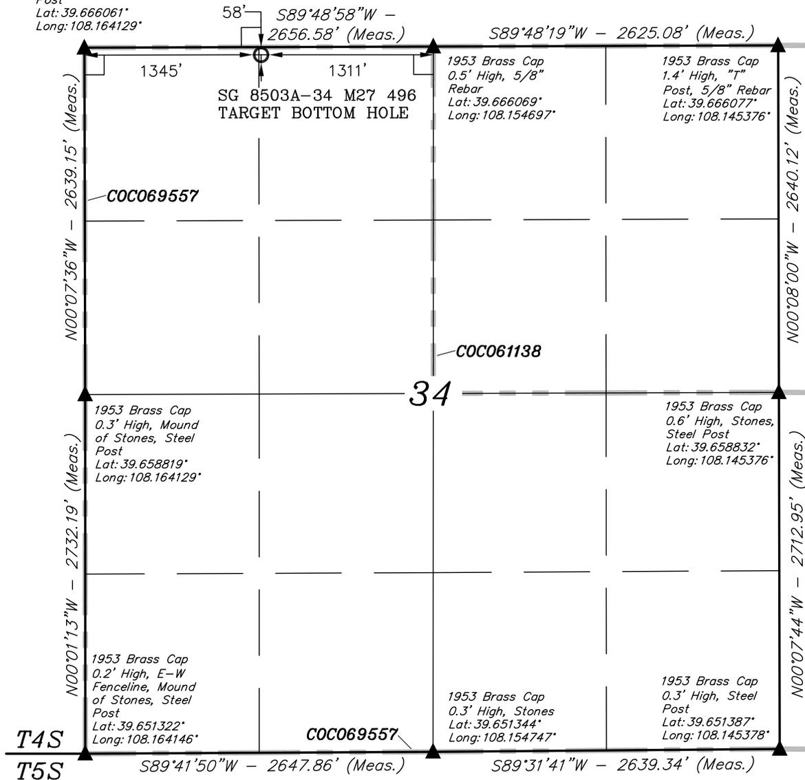
Well location, SG 8503A-34 M27 496 (TARGET BOTTOM HOLE), located as shown in the NE 1/4 NW 1/4 of Section 34, T4S, R96W, 6th P.M., Garfield County, Colorado.
