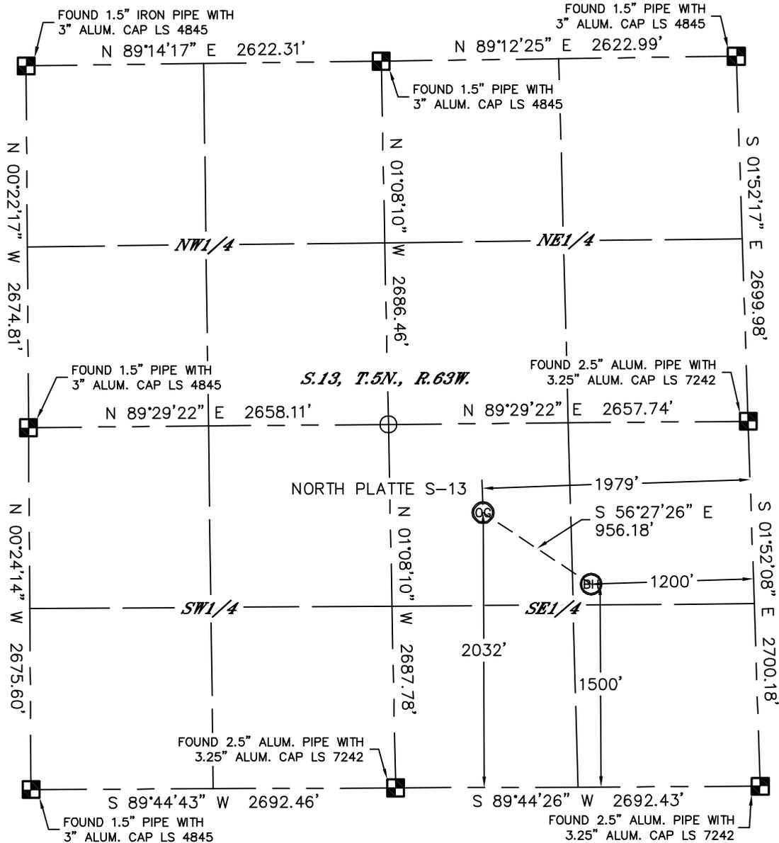
In accordance with a request from Keith Caplan with BONANZA CREEK ENERGY, INC. Lat40°, Inc. has determined the surface location of the NORTH PLATTE S-13 to be 2032' from the SOUTH line and 1979' from the EAST line and the bottom hole to be 1500' from the SOUTH line and 1200' from the EAST line as measured at right angles from the section lines of Section 13, Township 5 North, Range 63 West of the Sixth Principal Meridian, County of Weld, State of Colorado.
