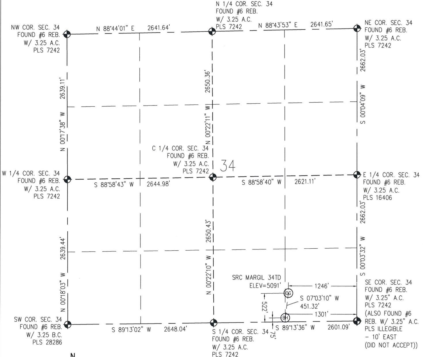
IN ACCORDANCE WITH A REQUEST FROM CRAIG RASMUSON - SYNERGY RESOURCES, BASELINE ENGINEERING CORP. HAS DETERMINED THE LOCATION OF THE SRC MARGIL 34TD TO BE 522' FSL AND 1,246' FEL, AS MEASURED AT NINETY (90) DEGREES FROM THE SECTION LINE OF SECTION 34, TOWNSHIP 4 NORTH, RANGE 68 WEST AND THE BOTTOM HOLE LOCATION TO BE 75' FSL AND 1,301' FEL OF SECTION 34, TOWNSHIP 4 NORTH, RANGE 68 WEST, 6TH PRINCIPAL MERIDIAN, WELD COUNTY, COLORADO.
