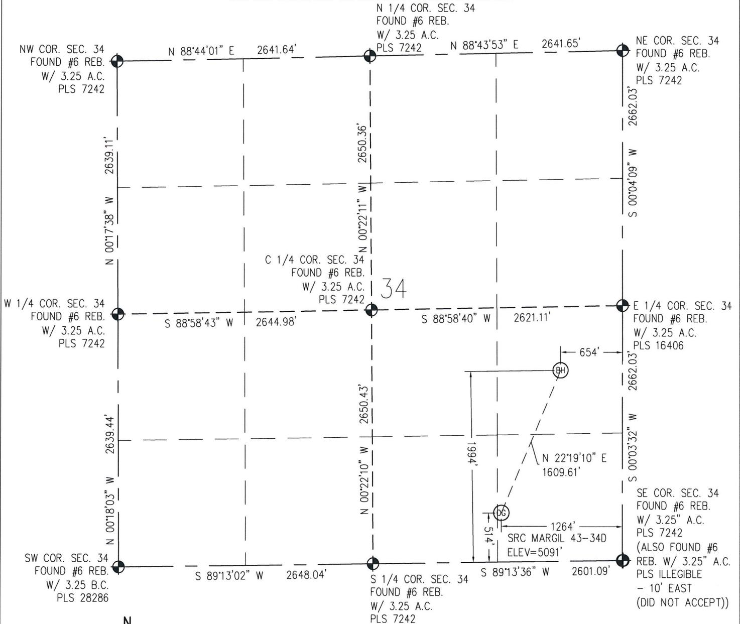
IN ACCORDANCE WITH A REQUEST FROM CRAIG RASMUSON - SYNERGY RESOURCES, BASELINE ENGINEERING CORP. HAS DETERMINED THE LOCATION OF THE SRC MARGIL 43-34D TO BE 514' FSL AND 1,264' FEL, AS MEASURED AT NINETY (90) DEGREES FROM THE SECTION LINE OF SECTION 34, TOWNSHIP 4 NORTH, RANGE 68 WEST AND THE BOTTOM HOLE LOCATION TO BE 1,994' FSL AND 654' FEL OF SECTION 34, TOWNSHIP 4 NORTH, RANGE 68 WEST, 6TH PRINCIPAL MERIDIAN, WELD COUNTY, COLORADO.
