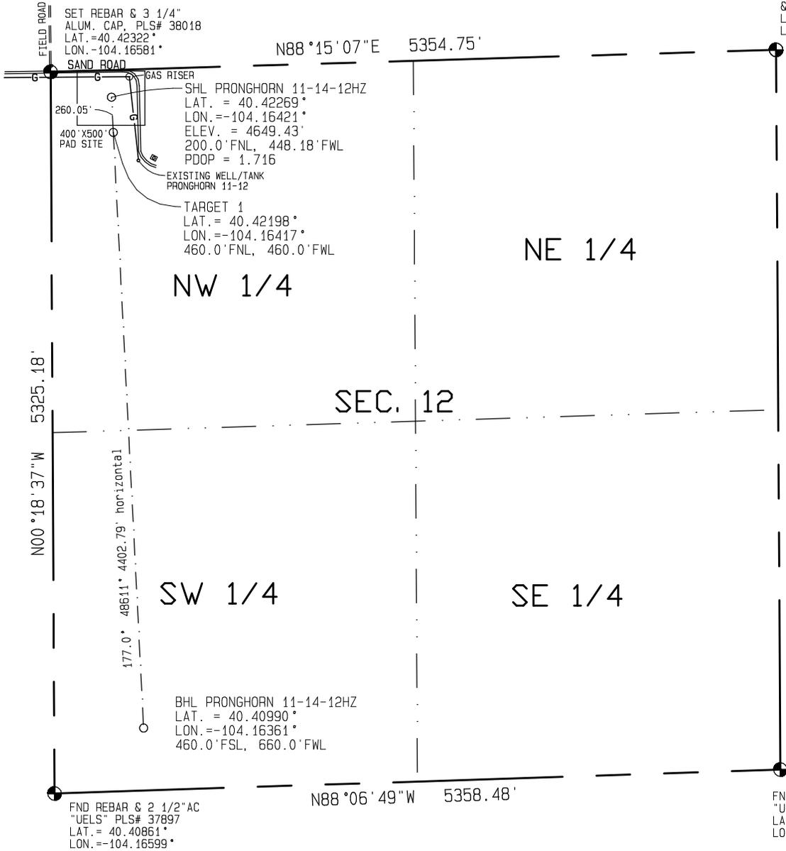
BASIS OF BEARINGS IS THE EAST LINE OF SEC. 12, T5N, R61W OF THE 6TH P.M. WELD COUNTY, CO. BEARS S00°20'48\"W BETWEEN SET MONUMENTS AS DETERMINED BY GPS (NAD 83)
