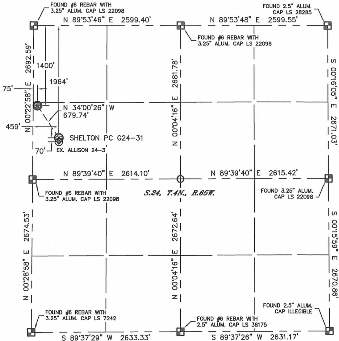
In accordance with a request from Ryan Hawkins with Noble Energy Inc. Lat40°, Inc. has determined the surface location of the SHELTON PC G24-31 to be 1964' from the NORTH line and 459' from the WEST line and the bottom hole to be 1400' from the NORTH line and 75' from the WEST line as measured at right angles from the section lines of Section 24, Township 4 North, Range 65 West of the Sixth Principal Meridian, County of Weld, State of Colorado.
