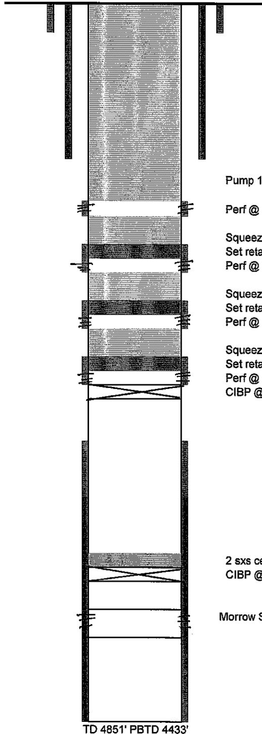
Pump 100 sxs cement down 4/12 csg and out to surface
