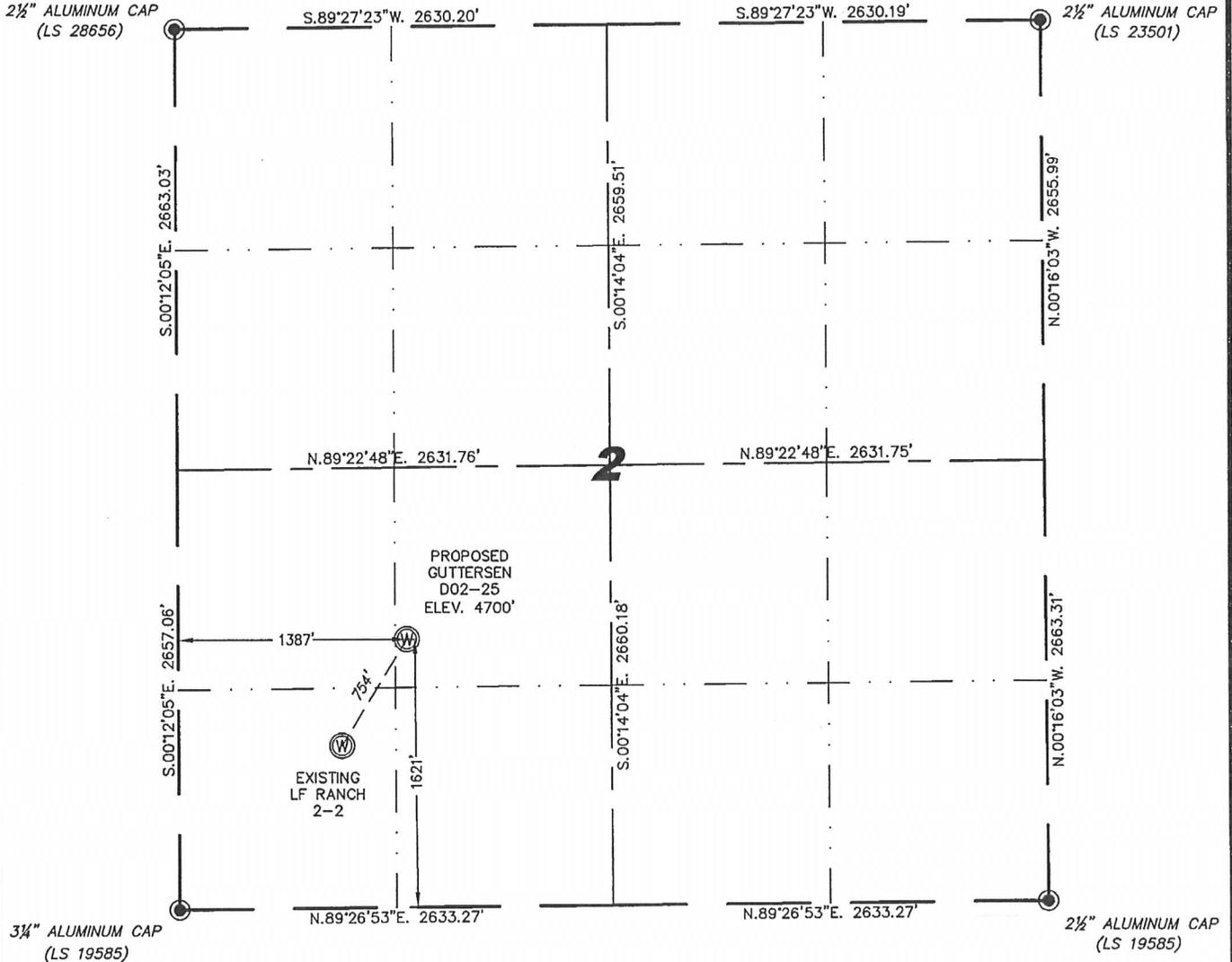
IN ACCORDANCE WITH A REQUEST FROM BRIAN DEROSE - NOBLE ENERGY INC, STEIL SURVEYING SERVICES, LLC HAS DETERMINED THE LOCATION OF THE GUTTERSEN D02-25 WELL TO BE 1621' FSL, 1387' FWL, AS MEASURED AT NINETY (90) DEGREES FROM THE SECTION LINES, SECTION 2, TOWNSHIP 3 NORTH, RANGE 64 WEST, 6TH PRINCIPLE MERIDIAN, WELD COUNTY, COLORADO.
