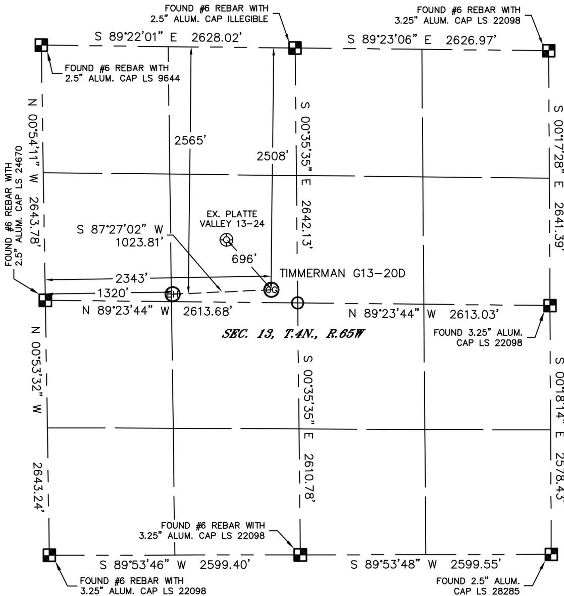
In accordance with a request from Nate McCorkell with Noble Energy Inc. Lat40°, Inc. has determined the surface location of the TIMMERMAN G13-20D to be 2508' from the NORTH line and 2343' from the WEST line and the bottom hole to be 2565' from the NORTH line and 1320' from the WEST line as measured at right angles from the section lines of Section 13, Township 4 North, Range 65 West of the Sixth Principal Meridian, County of Weld, State of Colorado.
