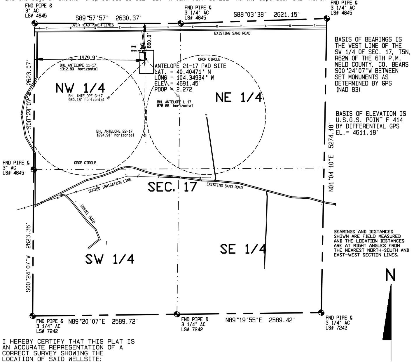
BASIS OF BEARINGS IS THE WEST LINE OF THE SW 1/4 OF SEC. 17, T5N, R62W OF THE 6TH P.M. WELD COUNTY, CO. BEARS S00°24'07"W BETWEEN SET MONUMENTS AS DETERMINED BY GPS (NAD 83)
