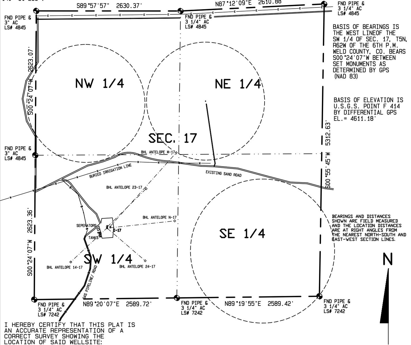
BASIS OF BEARINGS IS THE WEST LINE OF THE SW 1/4 OF SEC. 17, T5N, R62W OF THE 6TH P.M. WELD COUNTY, CO. BEARS S00°24'07\" W BETWEEN SET MONUMENTS AS DETERMINED BY GPS (NAD 83)
