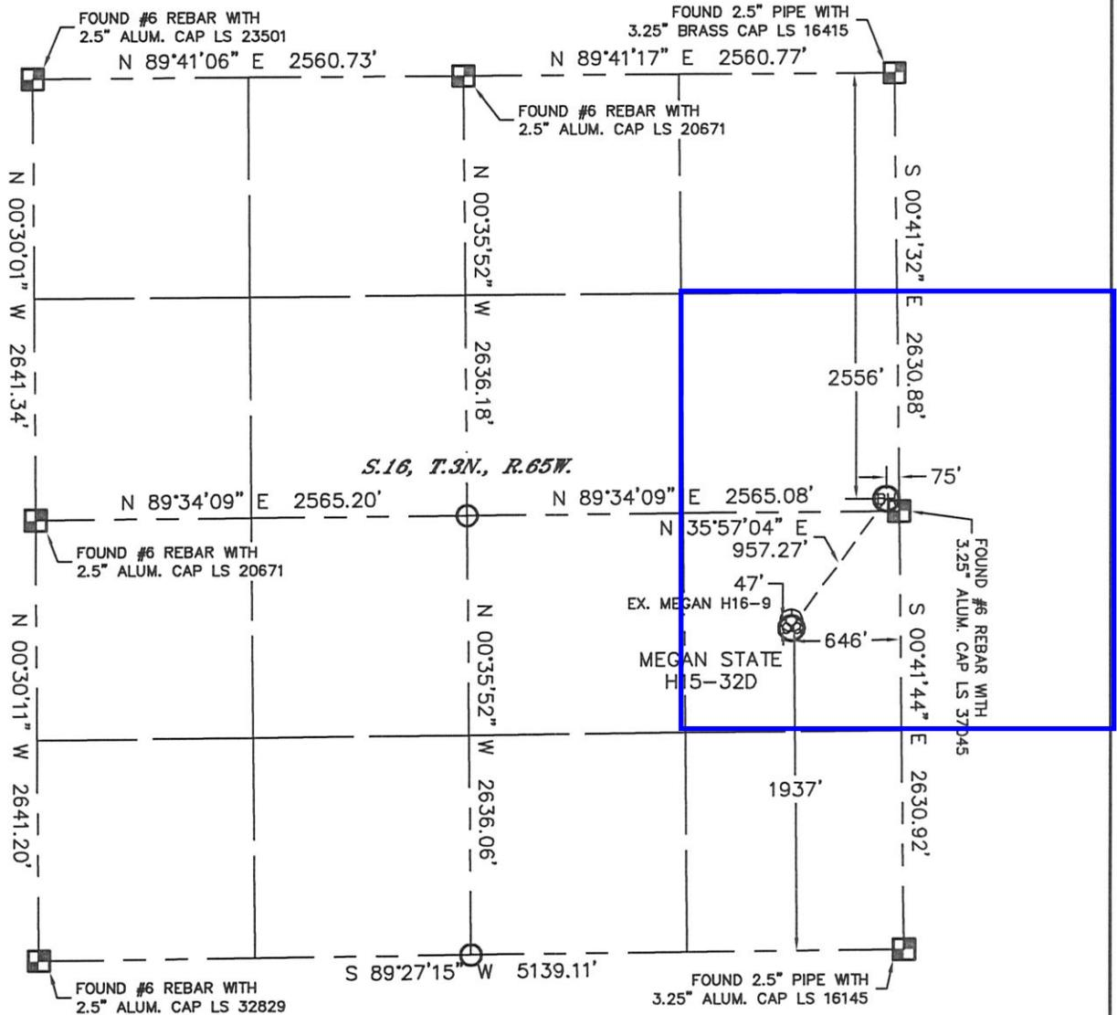
In accordance with a request from Ryan Hawkins with Noble Energy Inc. Lat40°, Inc. has determined the surface location of the MEGAN STATE H15-32D to be 1937' from the SOUTH line and 646' from the EAST line and the bottom hole to be 2556' from the NORTH line and 75' from the EAST line as measured at right angles from the section lines of Section 16, Township 3 North, Range 65 West of the Sixth Principal Meridian, County of Weld, State of Colorado.
