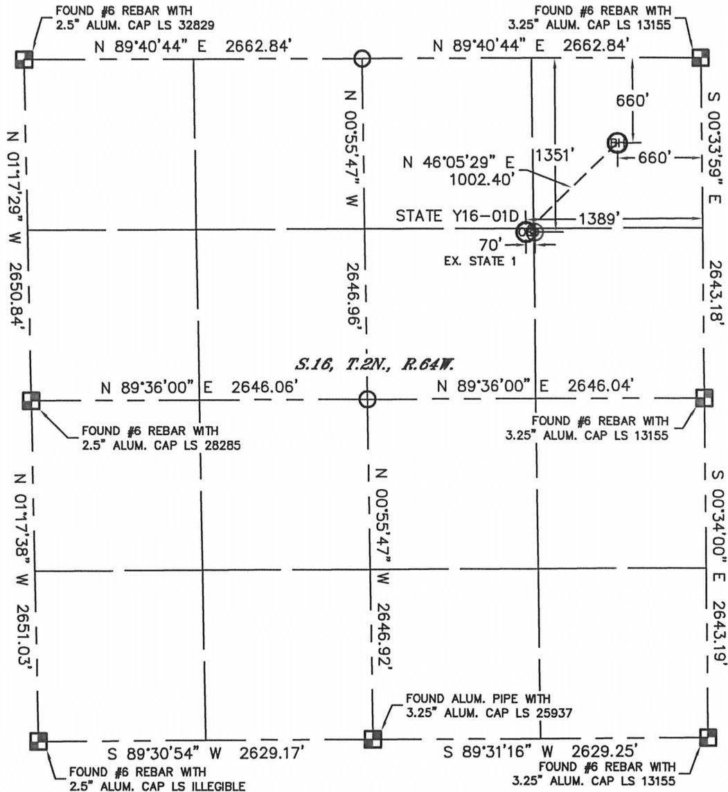
In accordance with a request from Matt Verbit with Noble Energy Inc., Lat40°, Inc. has determined the surface location of the STATE Y16-01D to be 1351' from the NORTH line and 1389' from the EAST line and the bottom hole to be 660' from the NORTH line and 660' from the EAST line as measured at right angles from the section lines of Section 16, Township 2 North, Range 64 West of the Sixth Principal Meridian, County of Weld, State of Colorado.
