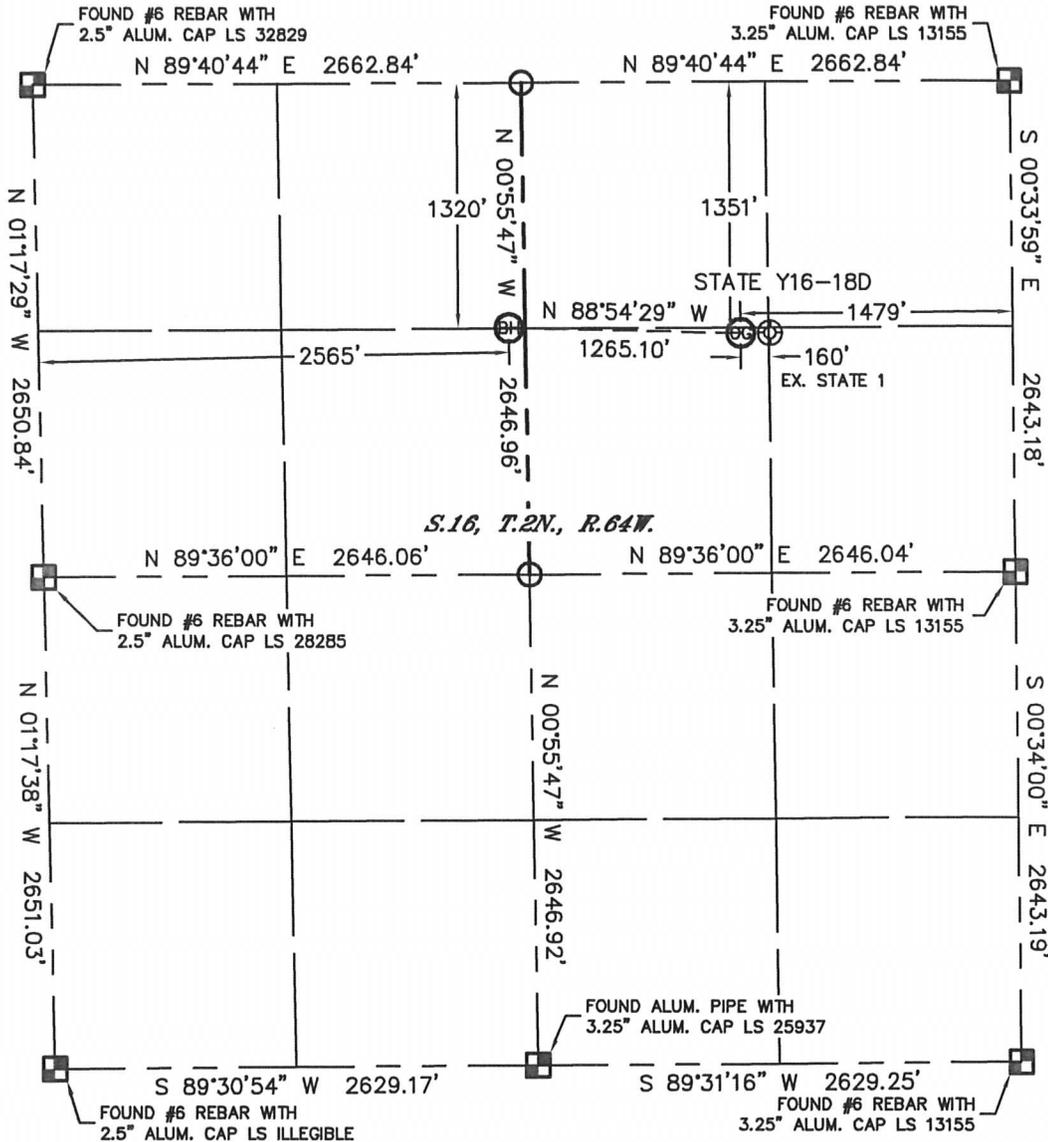
In accordance with a request from Matt Verbit with Noble Energy Inc., Lat40°, Inc. has determined the surface location of the STATE Y16-18D to be 1351' from the NORTH line and 1479' from the EAST line and the bottom hole to be 1320' from the NORTH line and 2565' from the WEST line as measured at right angles from the section lines of Section 16, Township 2 North, Range 64 West of the Sixth Principal Meridian, County of Weld, State of Colorado.
