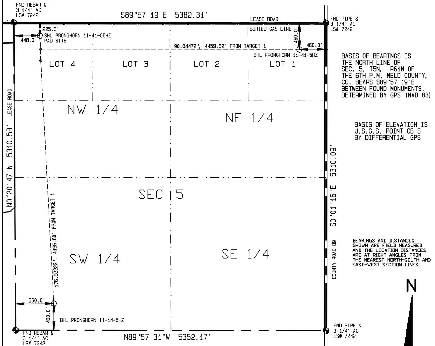
BASIS OF BEARINGS IS THE NORTH LINE OF SEC. 5, T5N, R61W OF THE 6TH P.M. WELD COUNTY, CO. BEARS S89°57'19\"E BETWEEN FOUND MONUMENTS. DETERMINED BY GPS (NAD 83)
