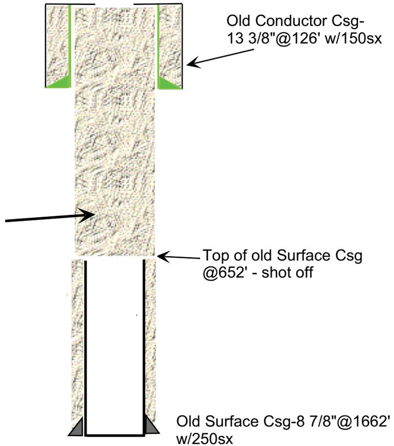
Could not get into old 8 7/8" surface casing. Top of old casing at 652' per impression block. Old casing shot off and top was crooked in hole.
