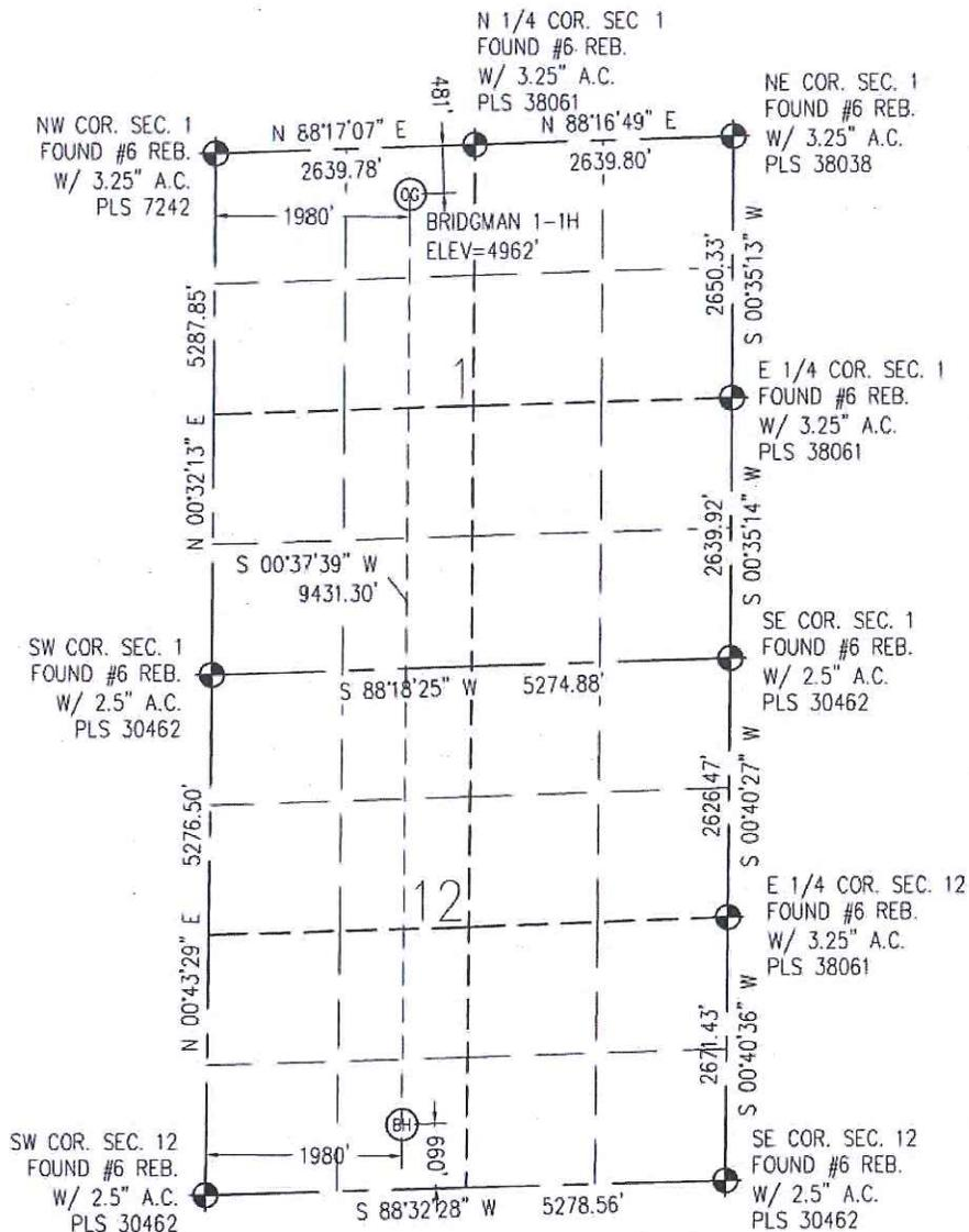
IN ACCORDANCE WITH A REQUEST FROM CHAD NEWBY - CONTINENTAL RESOURCES, BASELINE ENGINEERING CORP. HAS DETERMINED THE LOCATION OF THE BRIDGMAN 1-1H TO BE 481' FNL AND 1,980' FWL, AS MEASURED AT NINETY (90) DEGREES FROM THE SECTION LINE OF SECTION 1, TOWNSHIP 7 NORTH, RANGE 61 WEST AND THE BOTTOM HOLE LOCATION TO BE 660' FSL AND 1,980' FWL OF SECTION 12, TOWNSHIP 7 NORTH, RANGE 61 WEST, 6TH PRINCIPAL MERIDIAN, WELD COUNTY, COLORADO.
