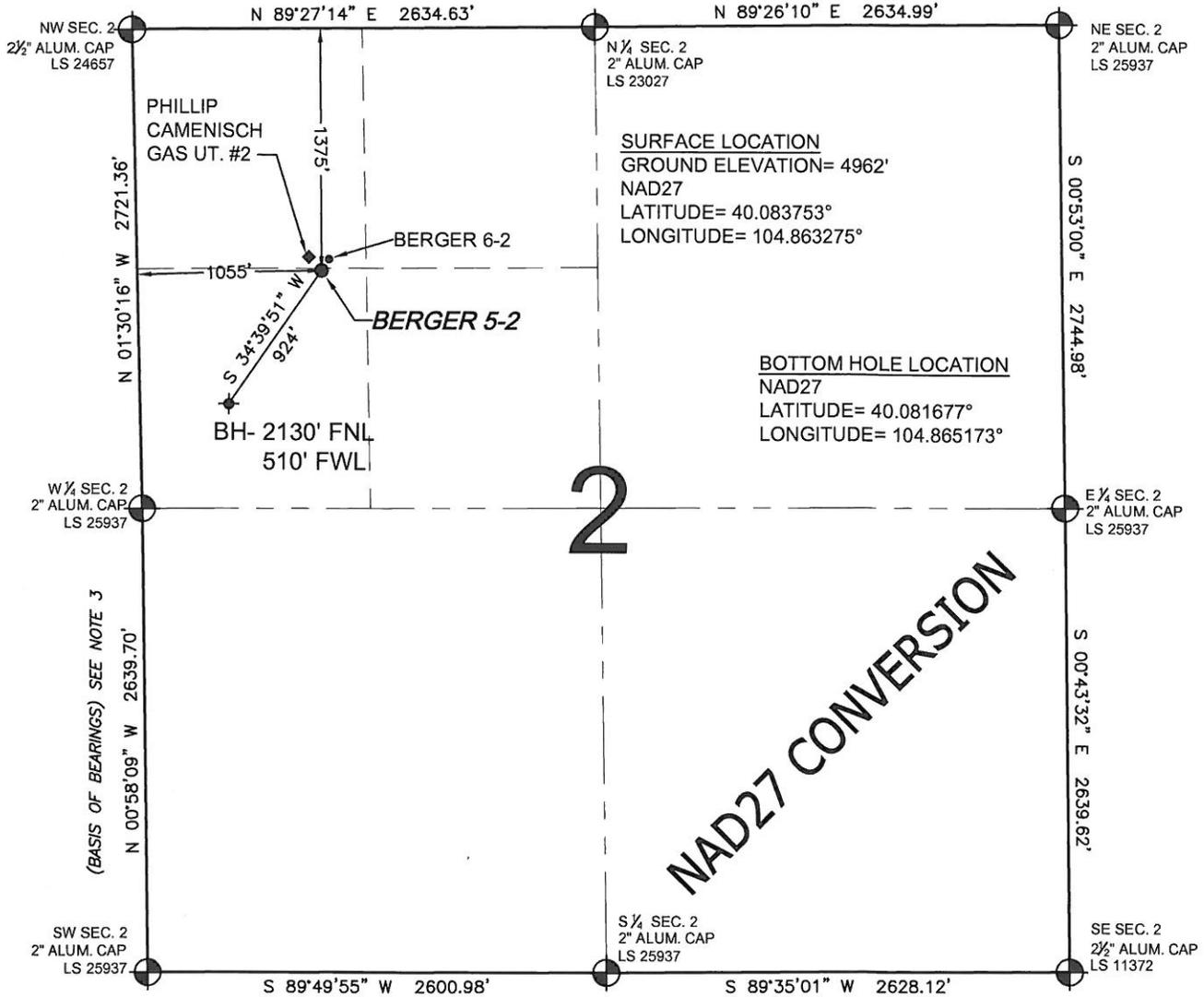
**WELL BERGER 5-2 TO BE LOCATED 1375' FNL AND 1055' FWL, SECTION 2, T1N, R67W OF THE 6th P.M.**
