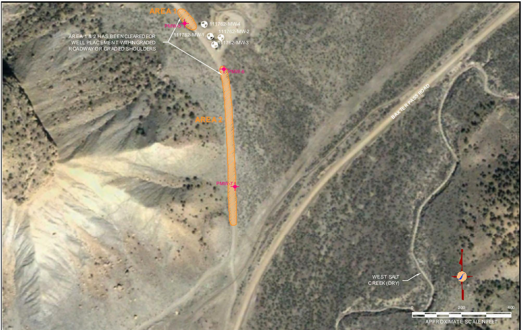
AREA 1 & 2 HAS BEEN CLEARED FOR WELL PLACEMENT WITHIN GRADED ROADWAY OR GRADED SHOULDERS
