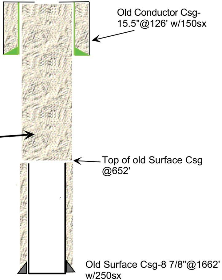
Could not get into old 8 7/8" surface casing. Top of old casing at 652'.
