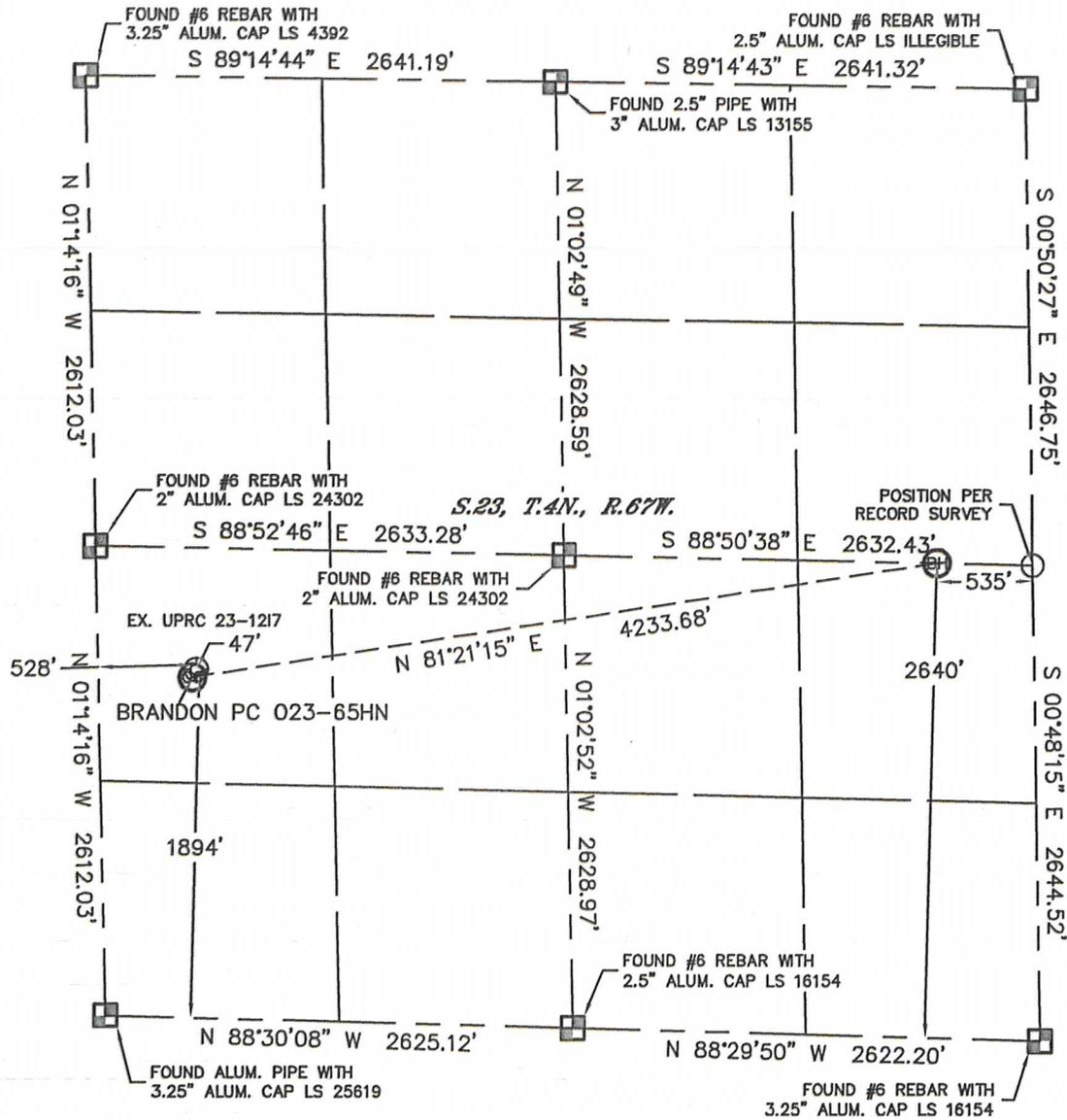
In accordance with a request from Erik Van Decar with Noble Energy Inc. Lat40°, Inc. has determined the surface location of the BRANDON PC 023-65HN to be 1894' from the SOUTH line and 528' from the WEST line and the bottom hole to be 2640' from the SOUTH line and 535' from the EAST line as measured at right angles from the section lines of Section 23, Township 4 North, Range 67 West of the Sixth Principal Meridian, Town of Milliken, County of Weld, State of Colorado.
