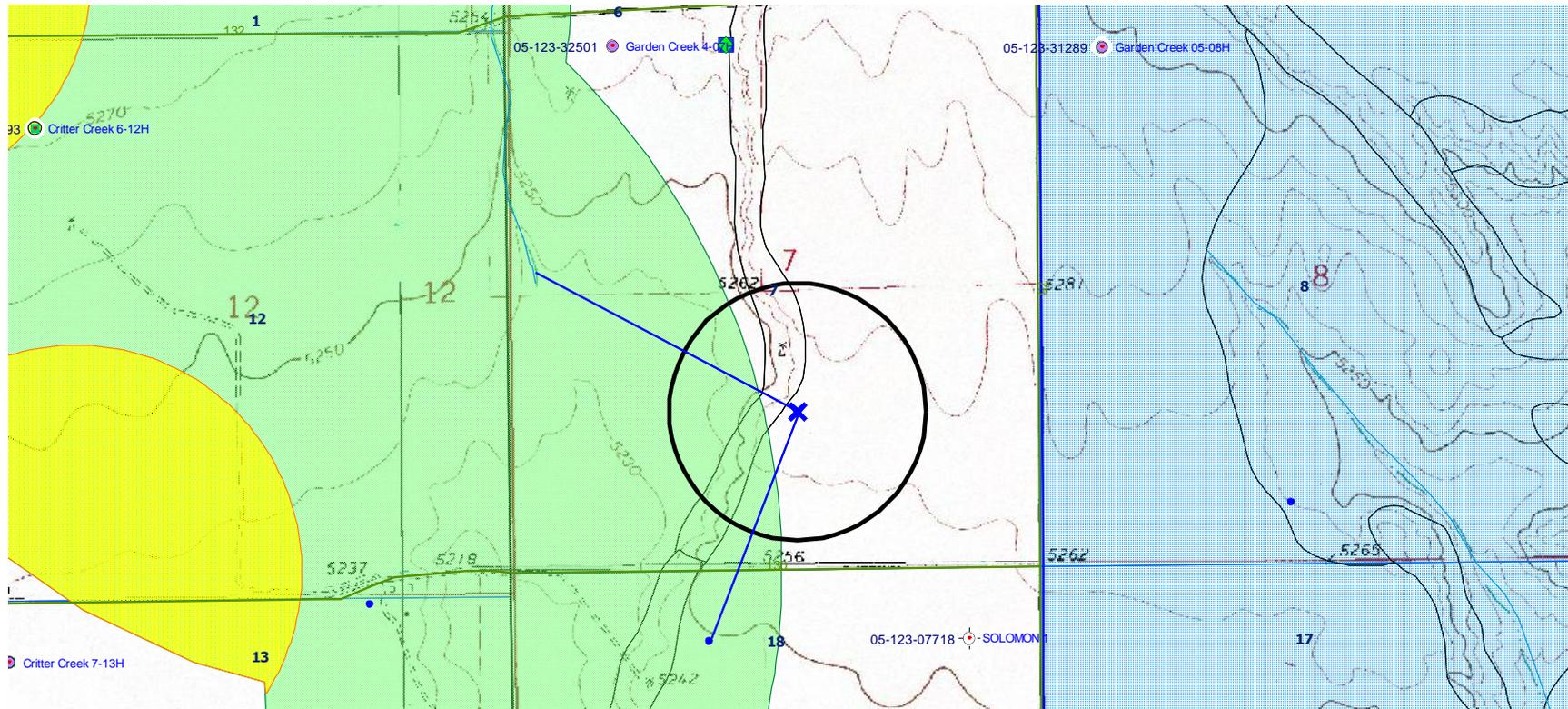
There is no surface water within 500 feet of the proposed Monitor well. Closest water well is to the south located within the NENW of section 18, T11N, R62W permit #12854.
