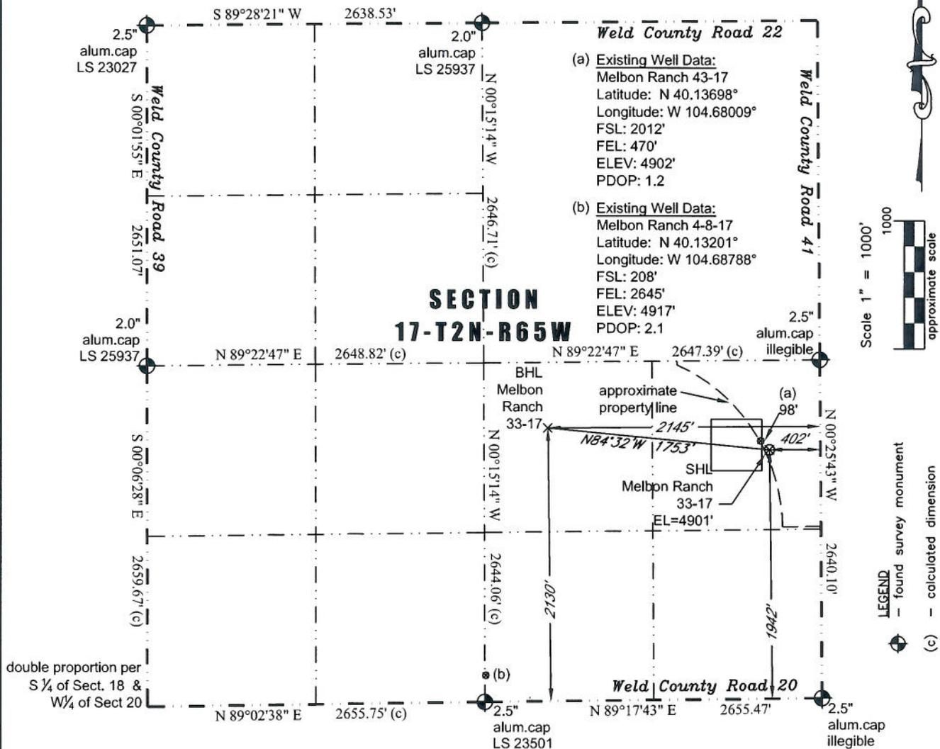
In accordance with a request from Jay Knutson of EnCana Oil & Gas (USA) Inc., PLS Group, LLC has determined the location of the **Melbon Ranch 33-17** well site to be SHL: 1942' FSL and 402' FEL, (BHL 2130' FSL and 2145' FEL), as measured at ninety (90) degrees from the section lines of Section 17, Township 2 North, Range 65 West of the 6th Principal Meridian, Weld County Colorado.
