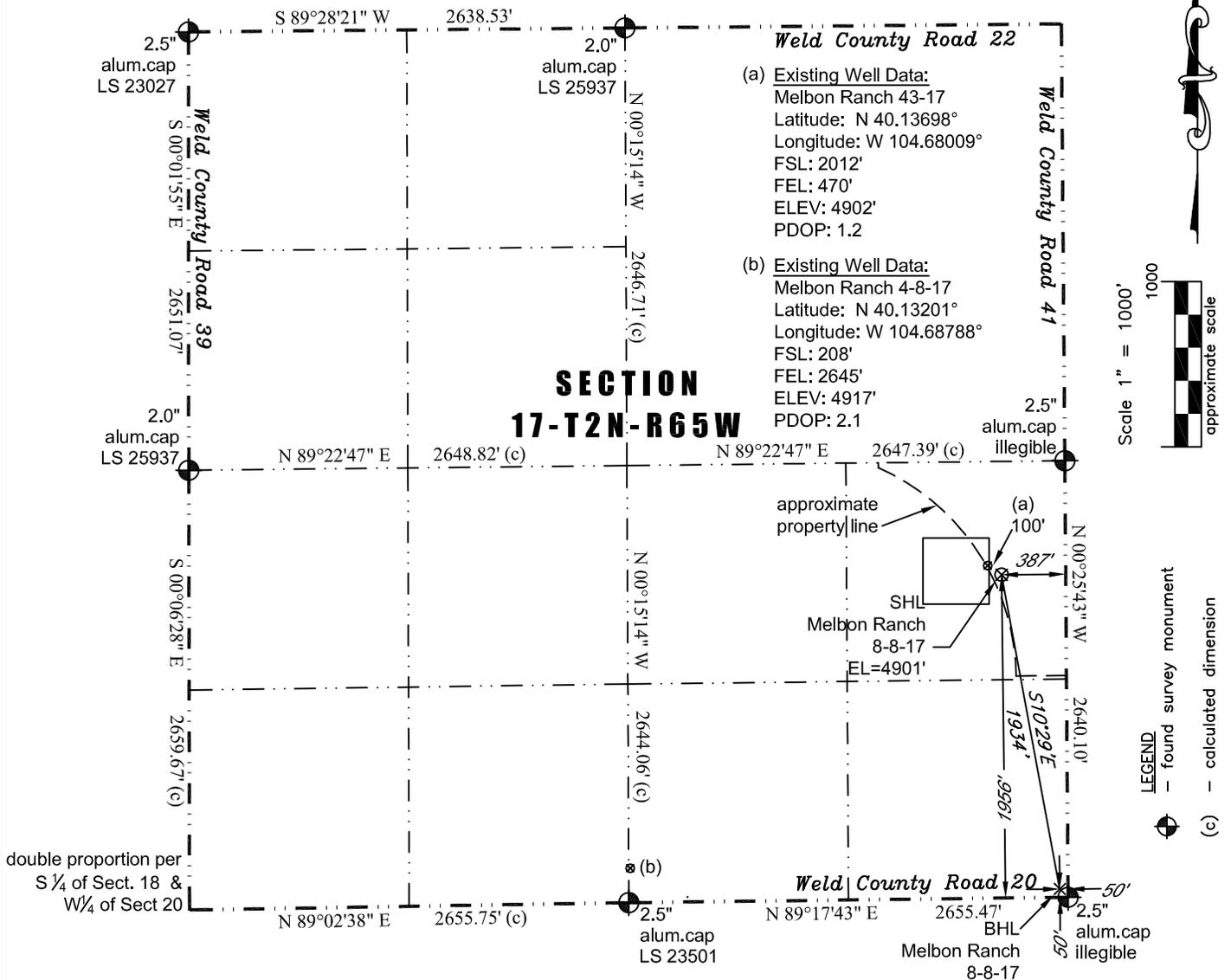
In accordance with a request from Jay Knutson of EnCana Oil & Gas (USA) Inc., PLS Group, LLC has determined the location of the **Melbon Ranch 8-8-17** well site to be SHL: 1956' FSL and 387' FEL, (BHL 50' FSL and 50' FEL), as measured at ninety (90) degrees from the section lines of Section 17, Township 2 North, Range 65 West of the 6th Principal Meridian, Weld County Colorado.
