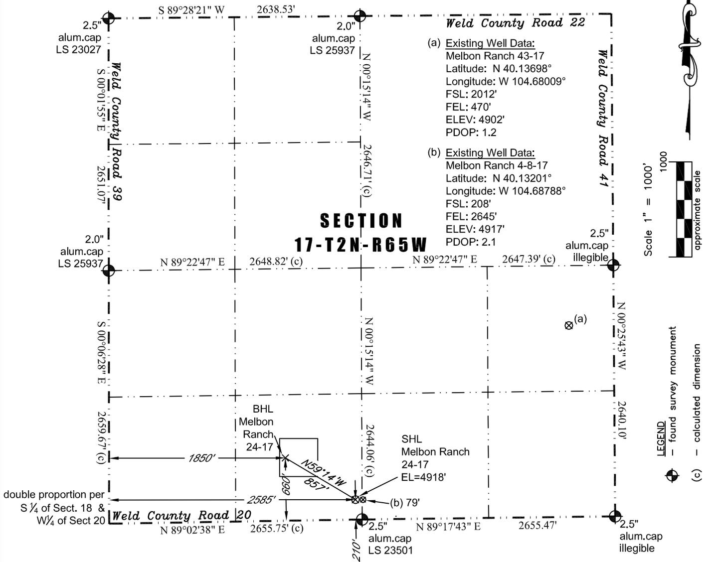
In accordance with a request from Jay Knutson of EnCana Oil & Gas (USA) Inc., PLS Group, LLC has determined the location of the **Melbon Ranch 24-17** well site to be SHL: 210' FSL and 2585' FWL, (BHL 660' FSL and 1850' FWL), as measured at ninety (90) degrees from the section lines of Section 17, Township 2 North, Range 65 West of the 6th Principal Meridian, Weld County Colorado.
