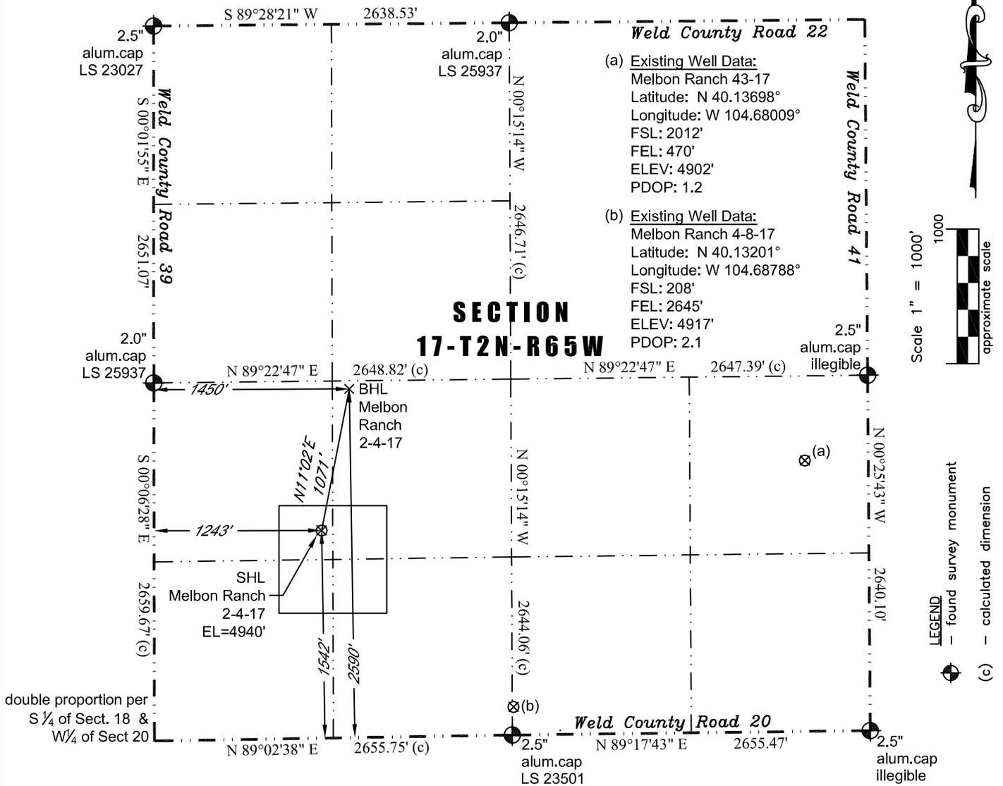
In accordance with a request from Jay Knutson of EnCana Oil & Gas (USA) Inc., PLS Group, LLC has determined the location of the **Melbon Ranch 2-4-17** well site to be SHL: 1542' FSL and 1243' FWL, (BHL 2590' FSL and 1450' FWL), as measured at ninety (90) degrees from the section lines of Section 17, Township 2 North, Range 65 West of the 6th Principal Meridian, Weld County Colorado.
