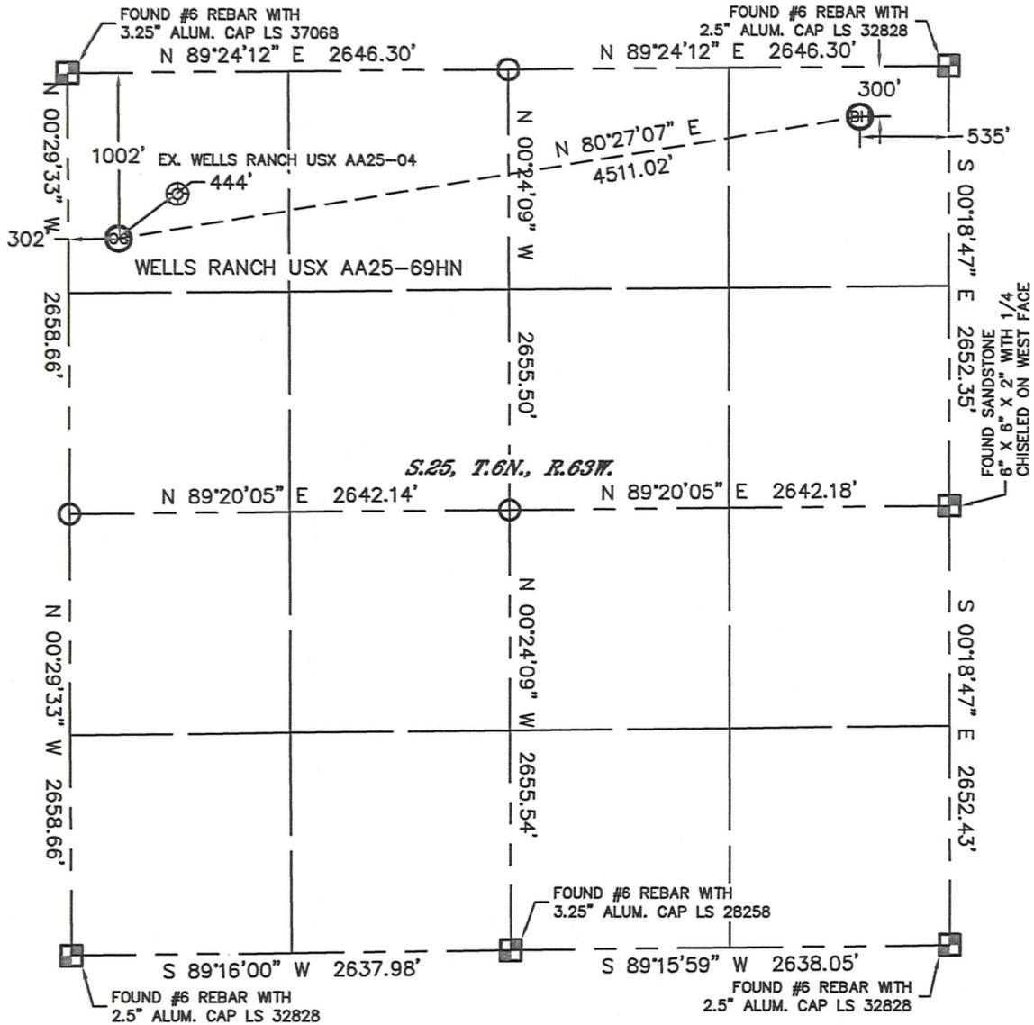
In accordance with a request from Sean Casper with Noble Energy Inc. Lat40°, Inc. has determined the surface location of the WELLS RANCH USX AA25-69HN to be 1002' from the NORTH line and 302' from the WEST line and the bottom hole to be 300' from the NORTH line and 535' from the EAST line as measured at right angles from the section lines of Section 25, Township 6 North, Range 63 West of the Sixth Principal Meridian, County of Weld, State of Colorado.
