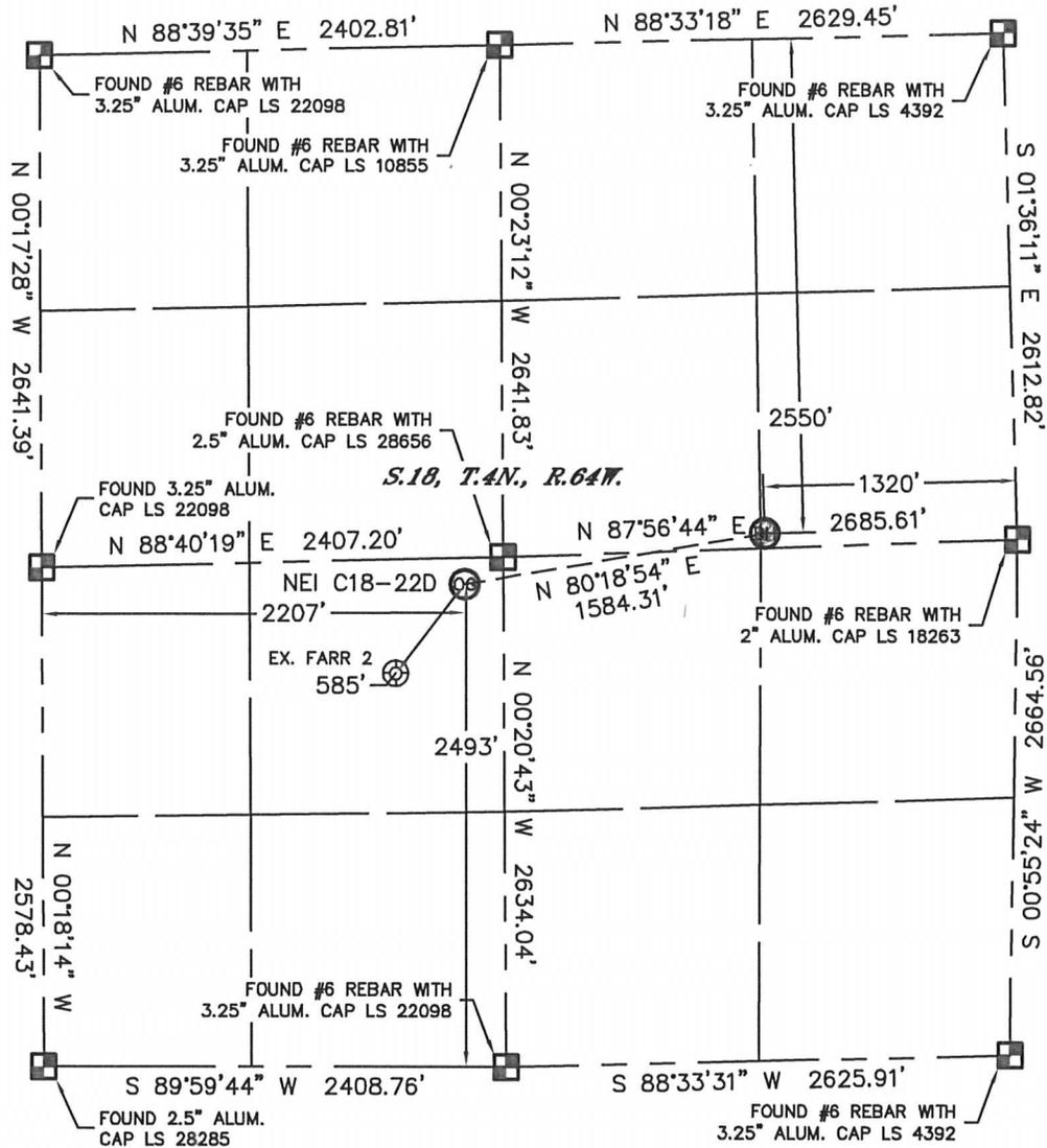
In accordance with a request from Matt Verbit with Noble Energy Inc. Lat40°, Inc. has determined the surface location of the NEI C18-22D to be 2493' from the SOUTH line and 2207' from the WEST line and the bottom hole to be 2550' from the NORTH line and 1320' from the EAST line as measured at right angles from the section lines of Section 18, Township 4 North, Range 64 West of the Sixth Principal Meridian, County of Weld, State of Colorado.
