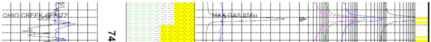
The high gas of the section was a maximum gas of 856 units and occurred at 7372'
