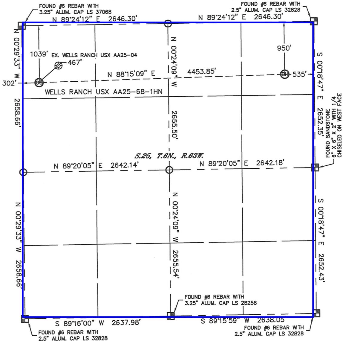
In accordance with a request from Sean Casper with Noble Energy Inc. Lat40°, Inc. has determined the surface location of the WELLS RANCH USX AA25-68-1HN to be 1039' from the NORTH line and 302' from the WEST line and the bottom hole to be 950' from the NORTH line and 535' from the EAST line as measured at right angles from the section lines of Section 25, Township 6 North, Range 63 West of the Sixth Principal Meridian, County of Weld, State of Colorado.
