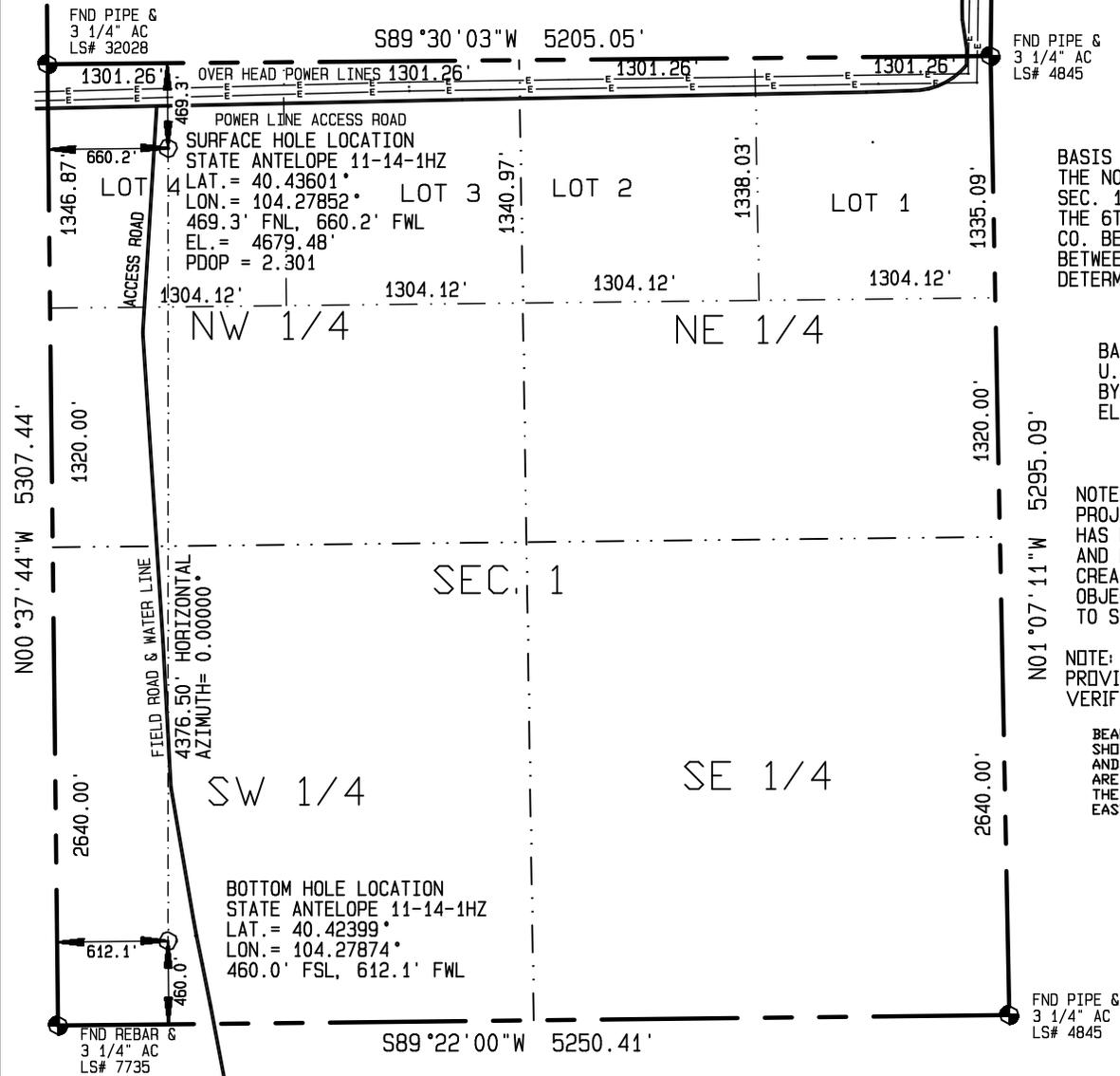
BASIS OF BEARINGS IS THE NORTH LINE OF SEC. 1, T5N, R62W OF THE 6TH P.M. WELD COUNTY, CO. BEARS N89°30'03"E BETWEEN FOUND MONUMENTS. DETERMINED BY GPS (NAD 83)
